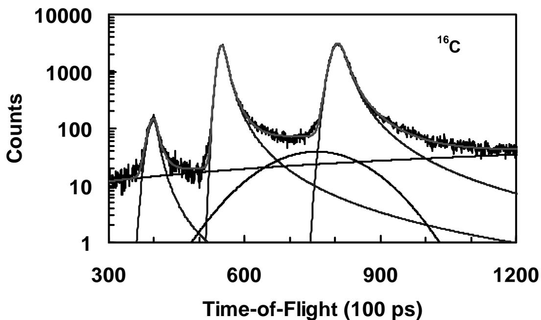
Figure 17 TOF spectrum of delayed neutrons detected by the neutron bar array for the decay of  $^{16}\text{C}$  showing the individual peaks, background and cumulative fit to the data.
