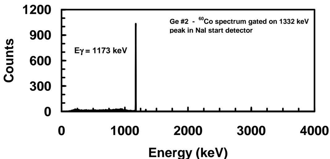
**Figure 44** <sup>60</sup>Co spectrum collected in Ge # 2 gated on the 1332 keV peak of the NaI start detector. The only notable transition is the coincident 1173 keV line.
