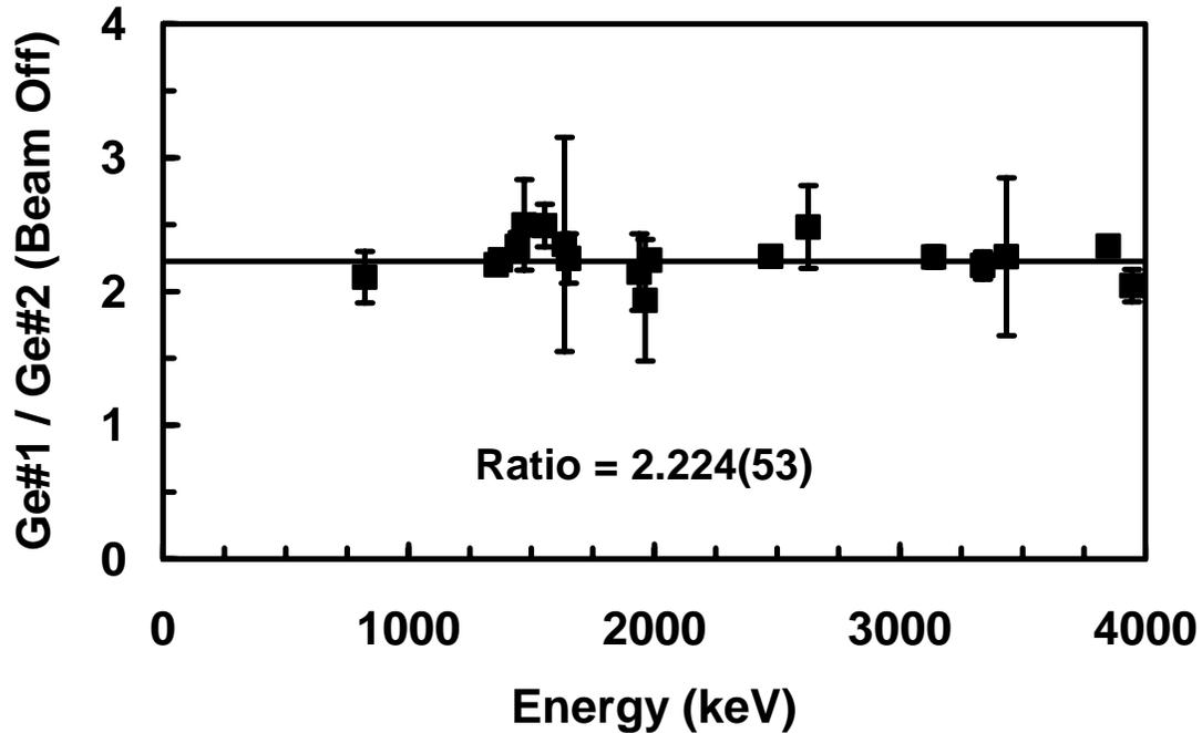
**Figure 40** A plot of the ratio of counts detected in Ge#1 to counts in Ge#2 during the beam-off period of the  $^{19}\text{N}$  experimental runs. The data are plotted at the ratio versus the energy of the gamma ray.
