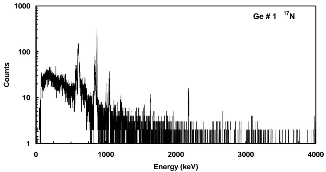
**Figure 34** Calibrated energy spectrum of events collected in germanium detector # 1 during the beam-off period of the <sup>17</sup>N runs. The data are plotted as intensity versus energy on a logarithmic scale.
