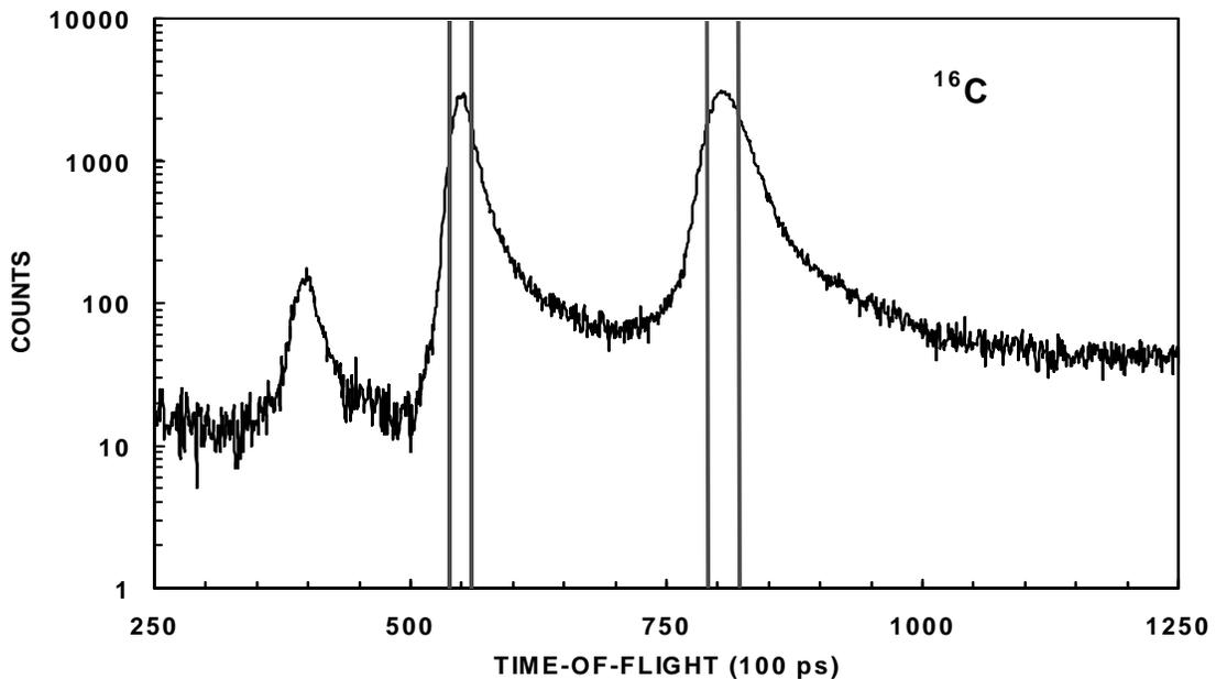
**Figure 11** Aggregate delayed neutron spectrum collected by the neutron bar array during the decay of  $^{16}\text{C}$ . Shown in red are the neutron gates used to reflect back onto the half-life spectrum for the dead-time analysis.
