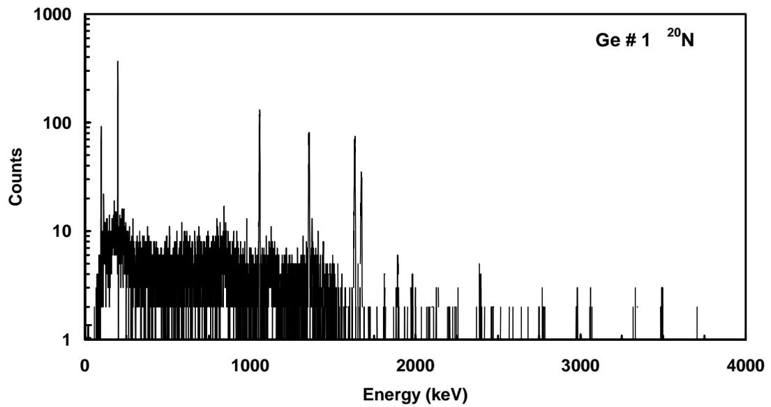
**Figure 38** Calibrated energy spectrum of events collected in germanium detector # 1 during the beam-off period of the  $^{20}\text{N}$  runs. The data are plotted as intensity versus energy on a logarithmic scale.
