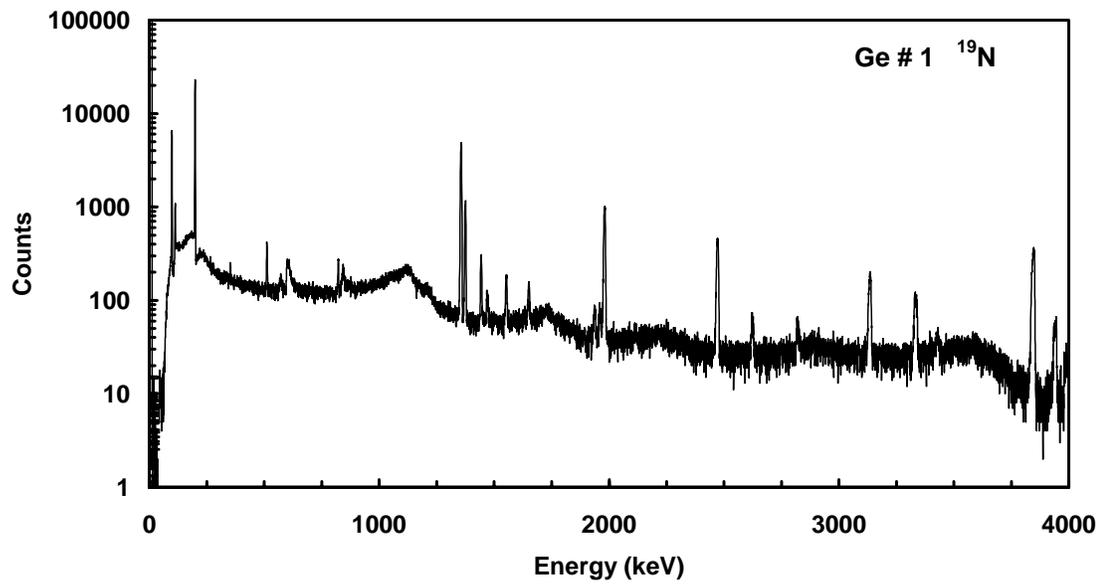
**Figure 36** Calibrated energy spectrum of events collected in germanium detector # 1 during the beam-off period of the <sup>19</sup>N runs. The data are plotted as intensity versus energy on a logarithmic scale.
