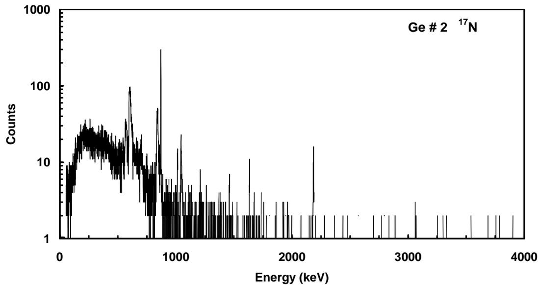
**Figure 35** Calibrated energy spectrum of events collected in germanium detector # 2 during the beam-off period of the <sup>17</sup>N runs. The data are plotted as intensity versus energy on a logarithmic scale.
