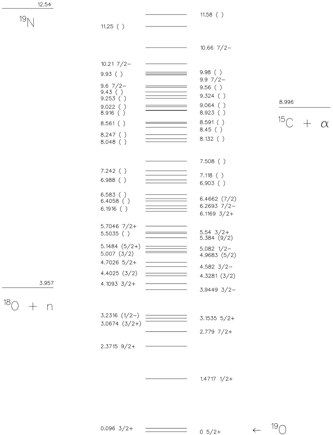
**Figure 1 Energy level diagram of the portion of the mass 19 system pertinent to the decay of  $^{19}\text{N}$ . The energies are given in MeV and are relative to the ground state of  $^{19}\text{O}$ .**
