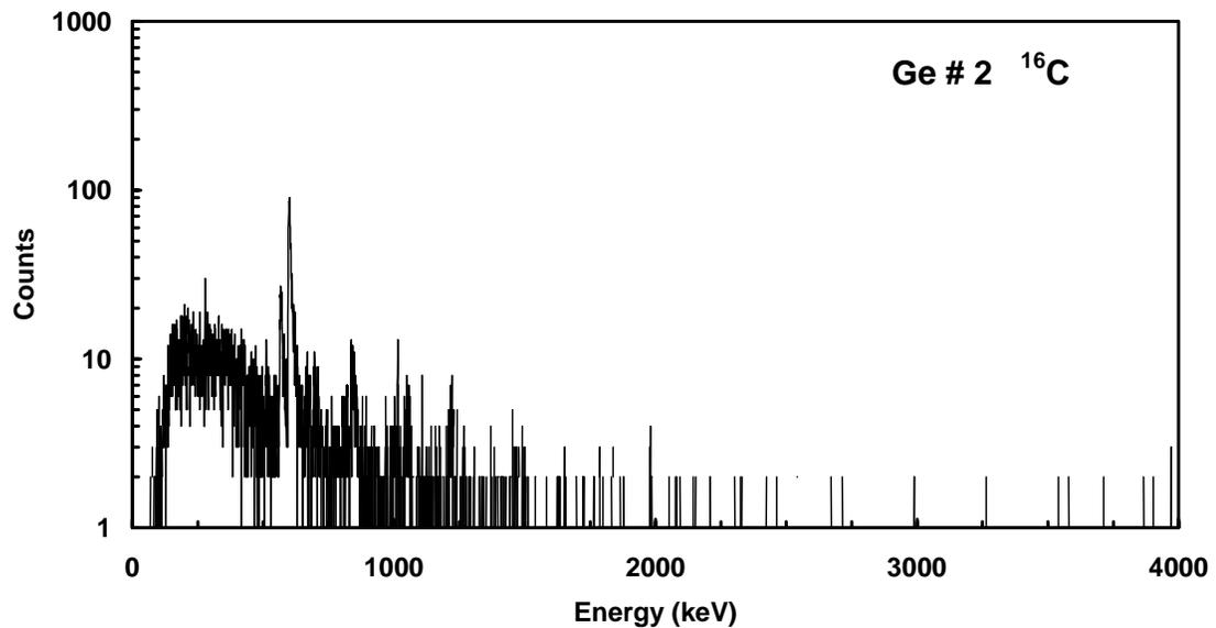
**Figure 33** Calibrated energy spectrum of events collected in germanium detector # 2 during the beam-off period of the  $^{16}\text{C}$  runs. The data are plotted as intensity versus energy on a logarithmic scale.
