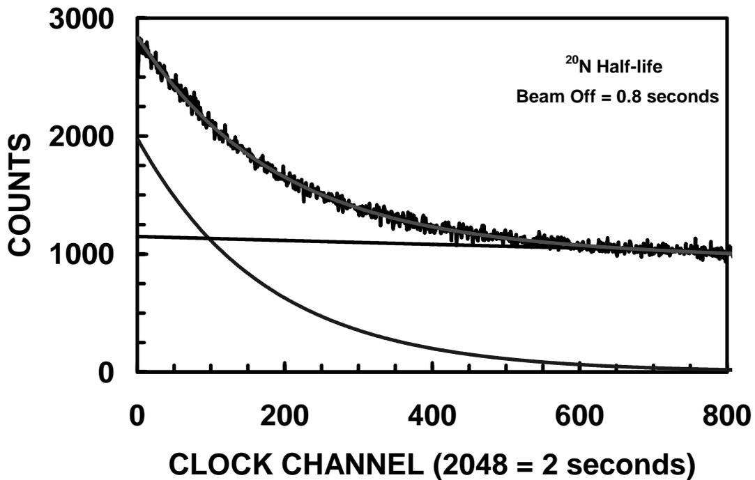
**Figure 10** Half-life fit for the  $^{20}\text{N}$  decay data recorded by the implantation scintillator and the real-time clock. This figure is the fit to the  $^{20}\text{N}$  decay measured with a beam off time of 0.8 seconds.
