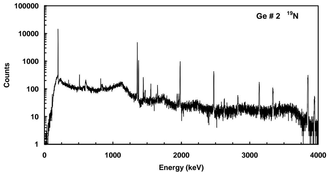
**Figure 37** Calibrated energy spectrum of events collected in germanium detector # 2 during the beam-off period of the <sup>19</sup>N runs. The data are plotted as intensity versus energy on a logarithmic scale.
