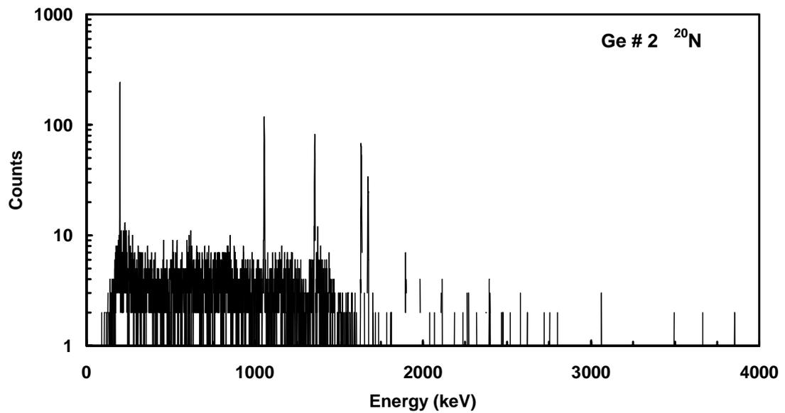
**Figure 39** Calibrated energy spectrum of events collected in germanium detector # 2 during the beam-off period of the  $^{20}\text{N}$  runs. The data are plotted as intensity versus energy on a logarithmic scale.
