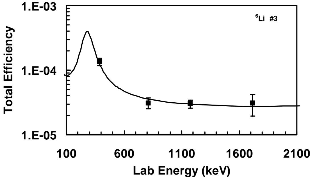
Figure 25 Calibration curve for the efficiency determination of lithium detector #3. The solid line represents the known neutron capture cross-sectional data on  ${}^6\text{Li}$  converted into relative efficiency and scaled to fit the data points measured.
