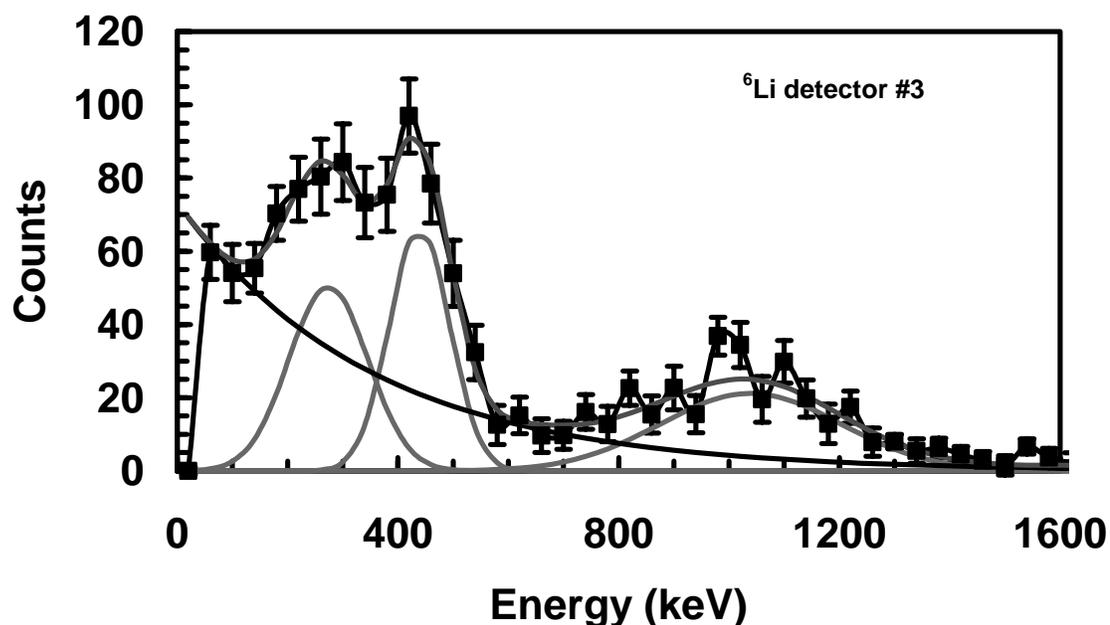
**Figure 29** Energy spectrum of delayed neutrons observed in lithium detector #3 during the decay of  $^{19}\text{N}$ . The width of the energy bins is 40 keV.
