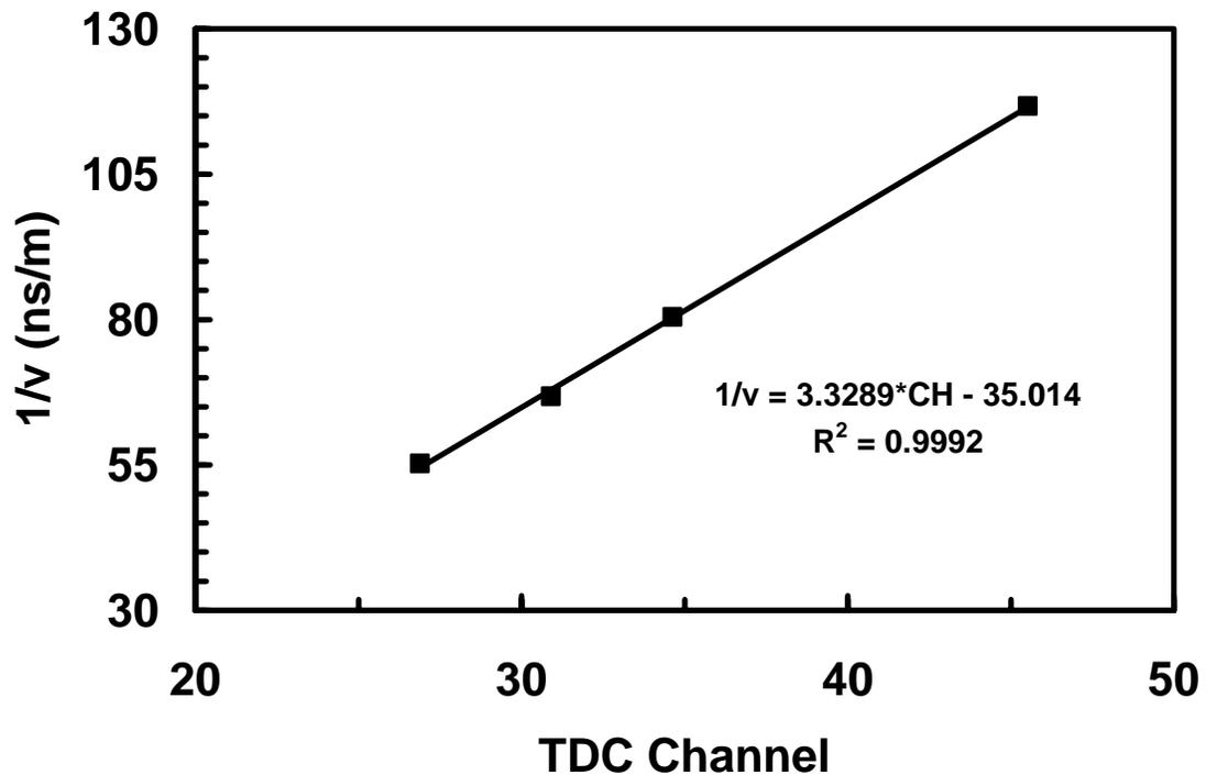
**Figure 24** Calibration curve of lithium detector #3 from the known delayed neutrons of  ${}^{16}\text{C}$  and  ${}^{17}\text{N}$ . The y-axis is in units of inverse velocity (ns/m) and is related to the neutron energy. The TDC was compressed to reflect 7 bits full-scale.
