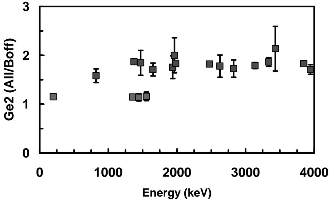
**Figure 41** The ratio of counts detected in Ge #2 at all times to counts detected during the beam off period plotted against gamma-ray energy. The colors indicate those gamma rays that appear to originate from the same source.
