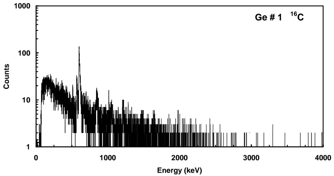
**Figure 32** Calibrated energy spectrum of events collected in germanium detector # 1 during the beam-off period of the  $^{16}\text{C}$  runs. The data are plotted as intensity versus energy on a logarithmic scale.
