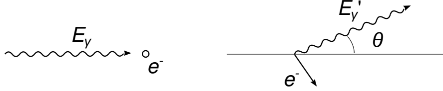
Figure 3.11: Schematic illustration of the Compton-scattering process.
