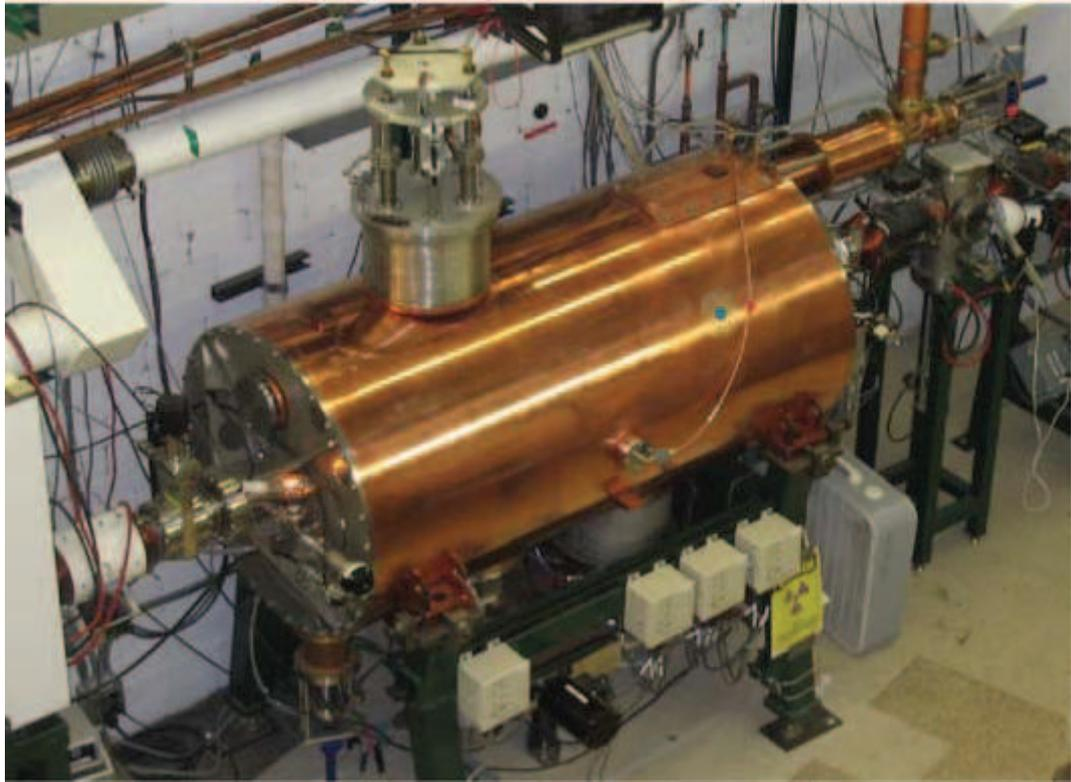
Figure 3.4: Photograph of the RF-kicker, installed in the S1/S2 vaults. The vacuum vessel is a cylinder made of copper-plated steel with an inner diameter of 0.9 m. The beam enters the cavity from the left. The end of the RF guide connected to the RF coupler is visible at the top right. Figure reproduced from [55].
