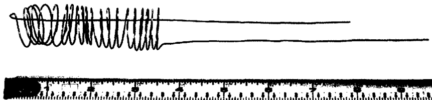
Figure 3.6: Heating element fabricated from tungsten wire using the mandrel shown in Figure 3.5. The wire used to fabricate the heating element pictured above was of diameter 7.62 \times 10^{-4} m (0.03").
