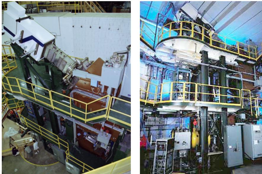
Figure 3.1: Focal plane detectors (left) and Superconducting Magnet (right) of the S800 spectrograph in the S3 vault at NSCL. Figure taken from [nsc].
