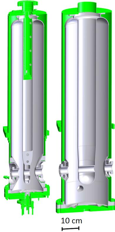
Figure 2.11: FRIB Quarter Wave Resonator designs.
