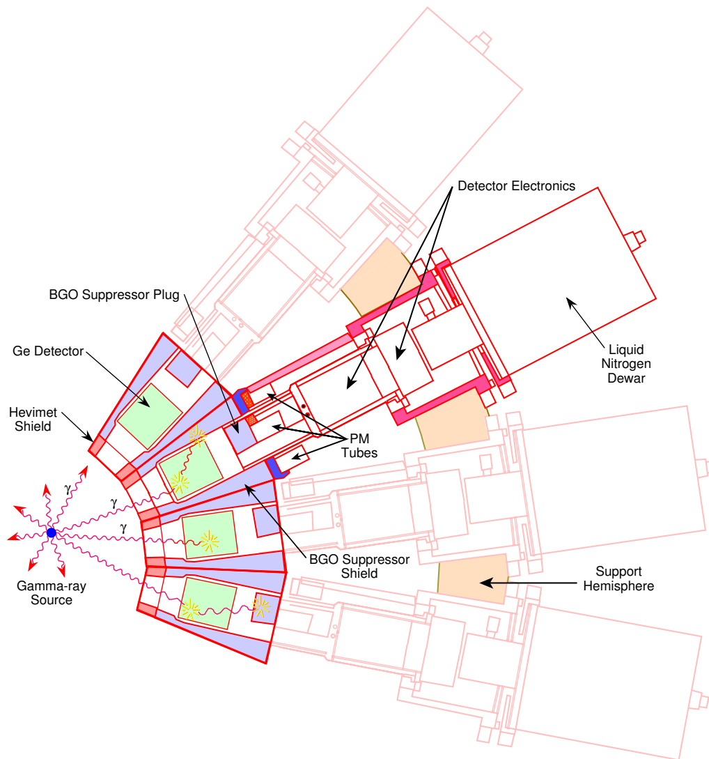
Figure 2.5: Schematic depiction of the layout of Gammasphere detector modules and of the types of interactions between \gamma rays and the detector material.
