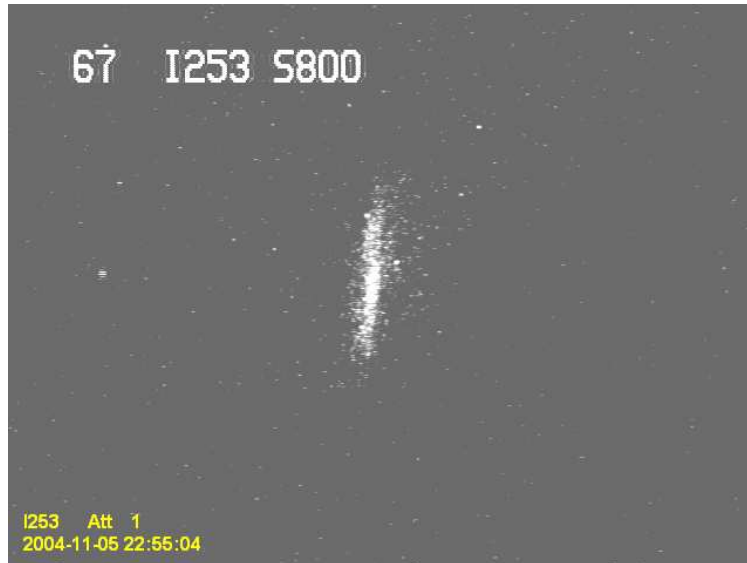
Figure 3.6: Typical triton secondary beam spot on a phosphor coated metal plate in the Large Scattering Chamber as seen by an image intensifying camera. The vertical dimension of the beam spot corresponds to 5 cm in the dispersive direction, and the horizontal dimension is a slightly distorted view of non-dispersive direction.
