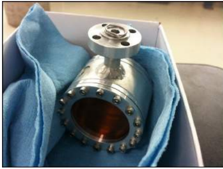
Figure 3.5: (Left) Photo of the target cell used to contain the Liquid Deuterium. The liquid drips down through the center hole seen on the target flange. The iridium seal can be seen surrounding it before being pressed. (Right) Drawing of the inner ring where the Kapton foil is glued. The ring is then clamped to the target by an outer ring visible in the left photo.
