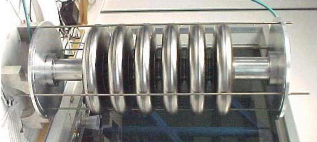
Figure 2.2. A 6-cell Niobium RF cavity.
