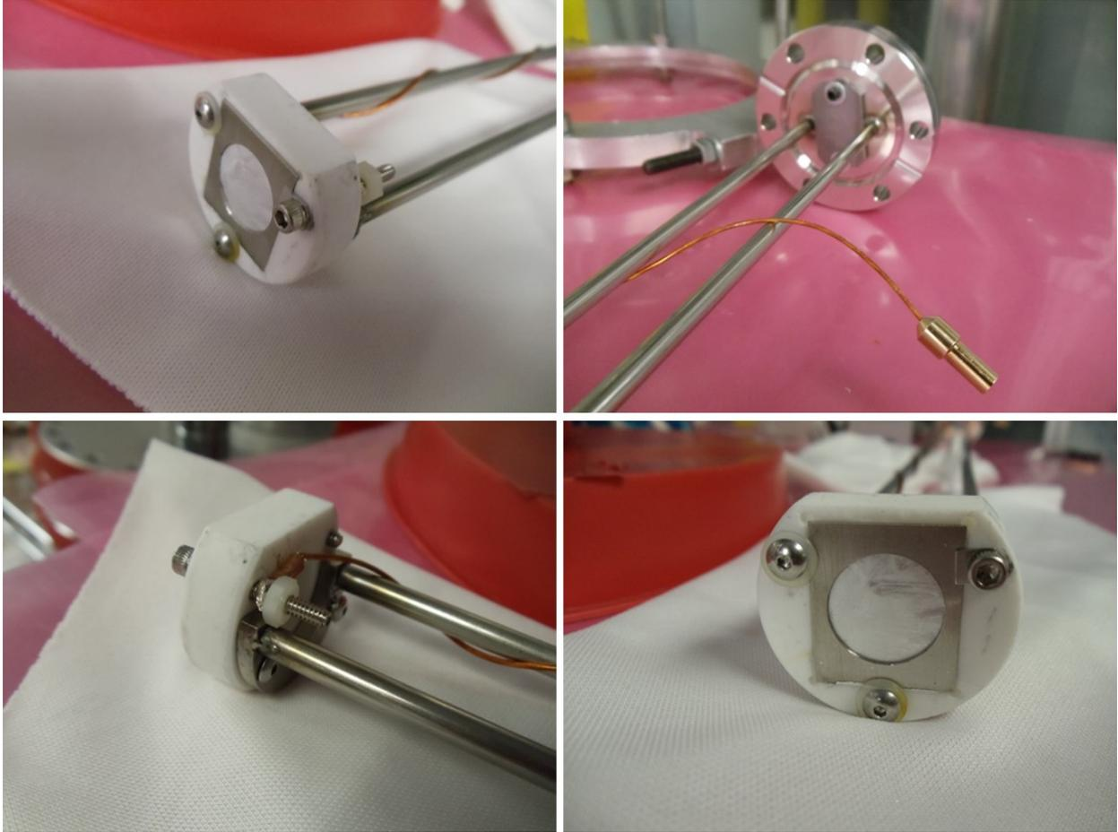
Figure 3.6 The target with the target holder apparatus for the CAESAR detector. The Al foil target was electrically isolated from the beam dump. By connecting a wire to the target frame, the current in the target and target frame can be read through a beam current monitor. The beam was collected on a tantalum sheet at the end of the beam-line.
