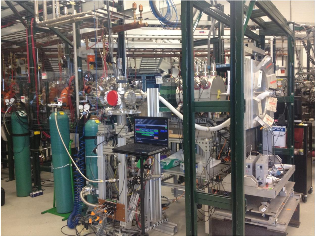
Figure 3.10 The SuN detector connected to the end of L-line extension beam line at ReA3.
