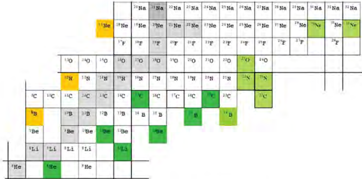
Figure 1.6 A focused view of the chart of nuclides is presented. Halo nuclei and potential halo nuclei are colored in. The valence nucleons in the orange colored nuclei are protons. The valence nucleons in the green colored nuclei are neutrons. The lighter shades of green are nuclei for which enhanced interaction cross sections have been measured. Darker shades of green are those nuclei for which both enhanced cross sections and narrow momenta distributions have been measured. Figure and discussion are from [26].
