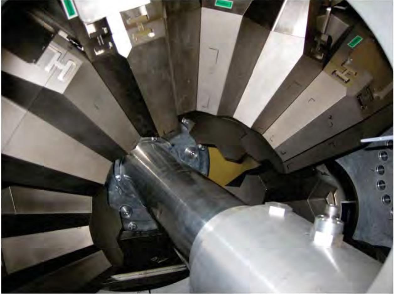
Figure 3.8 The GREINA setup used in the ^{27}\text{Ne} experiment in March 2016 is shown. Nine GREINA detectors were used in the experiment, which are arrayed around the beam pipe for the TRIPLEX plunger.
