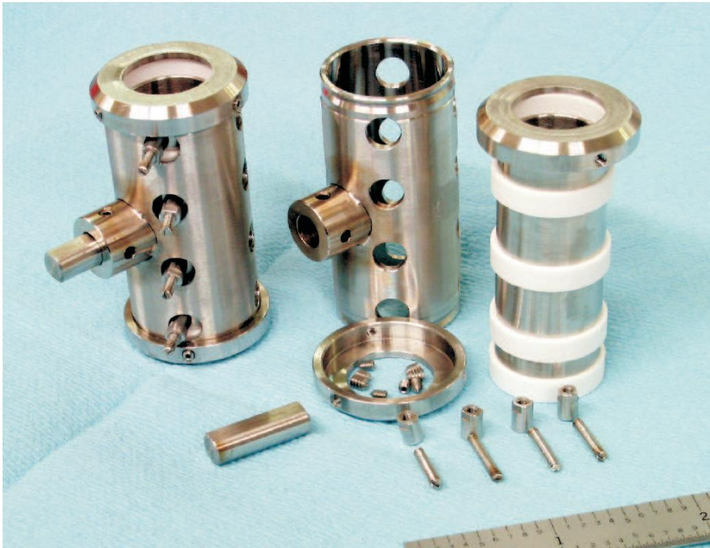
Figure 5.10: Photograph of Faraday cup during assembly
