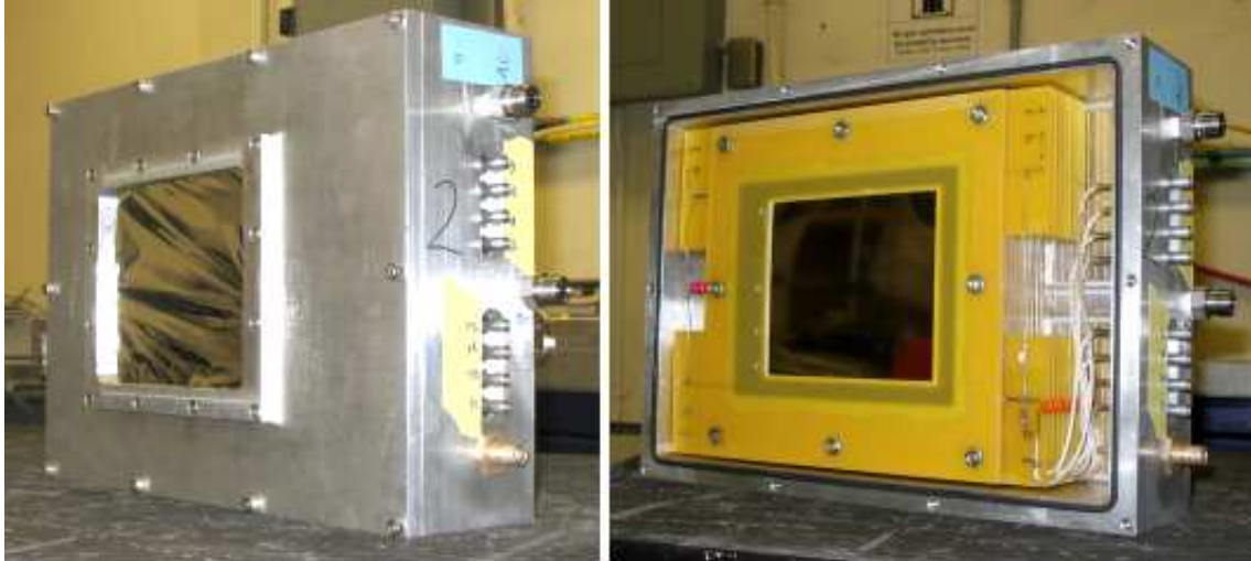
Figure 5.3: Photograph of one timing PPAC. The left panel shows the detector as it is used in the experiment, showing a pressure window. The right panel shows the inside of the detector with the stack of G10 boards.
