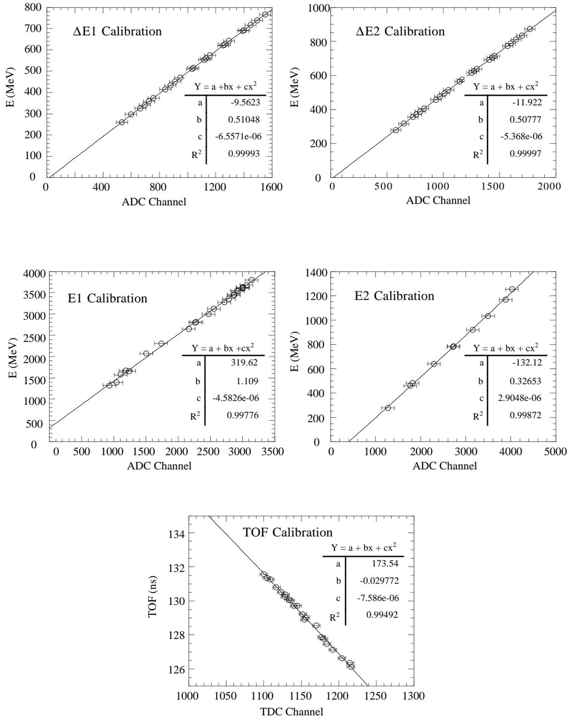
**FIGURE 3.5:** Energy and time calibrations for the detectors during the  $^{86}\text{Kr}$  fragmentation experiment.
