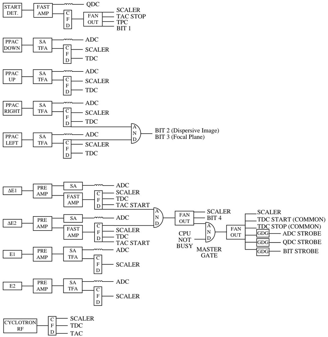
**FIGURE 3.2:** A schematic diagram of the electronic setup that was used during the fragmentation experiments.
