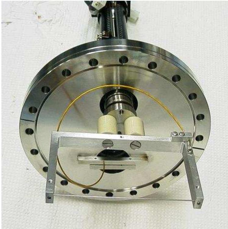
Figure 4.29: One of the two vertical scanning wire monitors. The wire holder in the monitor is wider than that in the horizontal wire monitors.
