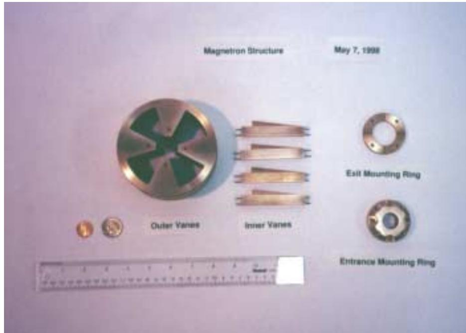
**Figure 77. Components of the magnetron section before assembly.**
