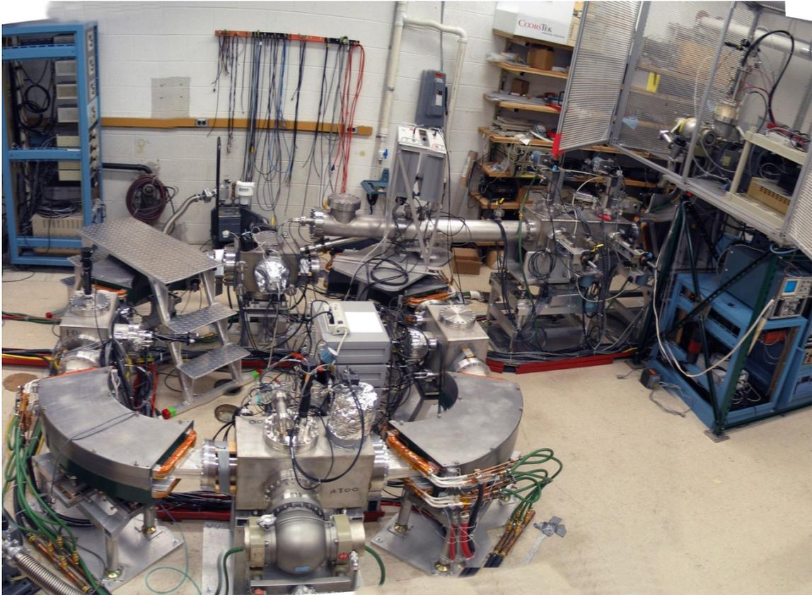
Figure 1: Picture of the Small Isochronous Ring (SIR).
