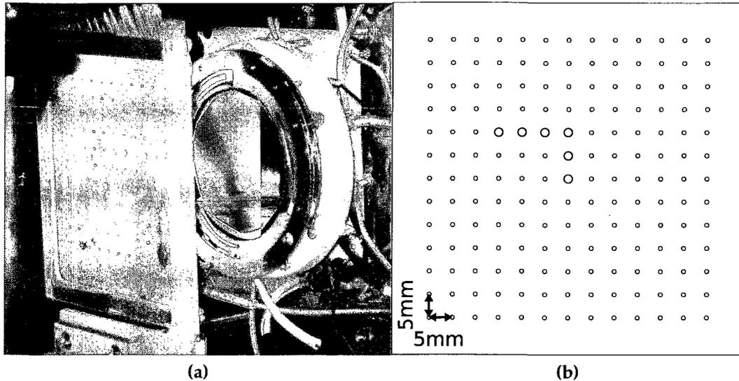
**Figure 3.15** – (a) Photograph of a rear view of the inserted MCP 1 calibration mask and MCP 1 detector. The beam enters from the right of photograph. (b) Schematic drawing of the MCP mask. All holes are separated by 5 mm. The diameter of the smaller holes is 1 mm while the larger holes that make up the L pattern are 2 mm.
