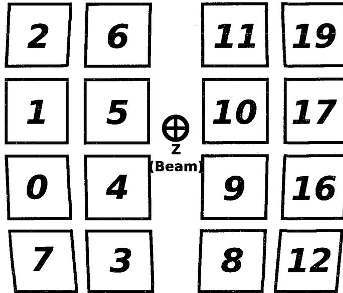
Figure 2.11 – HiRA telescope positions and their ID labels.
