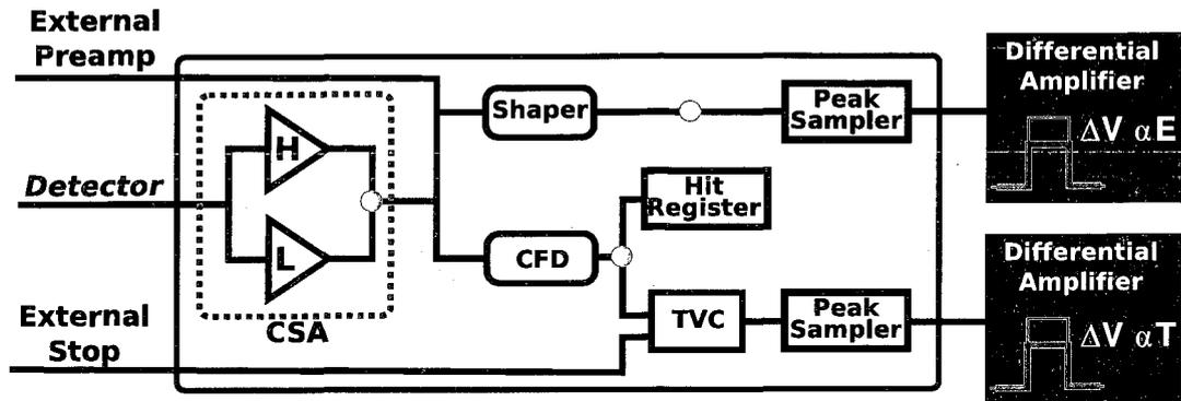
Figure 2.13 – Block diagram of a single channel of the HINP16C ASIC chip.
