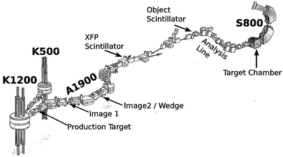
**Figure 2.3** – Schematic rendering of the coupled cyclotrons, A1900 fragment separator, and beamline to the S800. HiRA and the MCP tracking system are located inside the target chamber.
