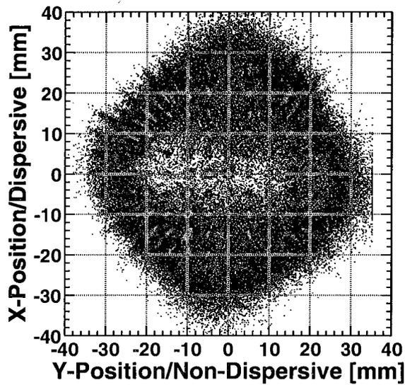
(a) MCP 0  $\alpha$ -source mask calibration
