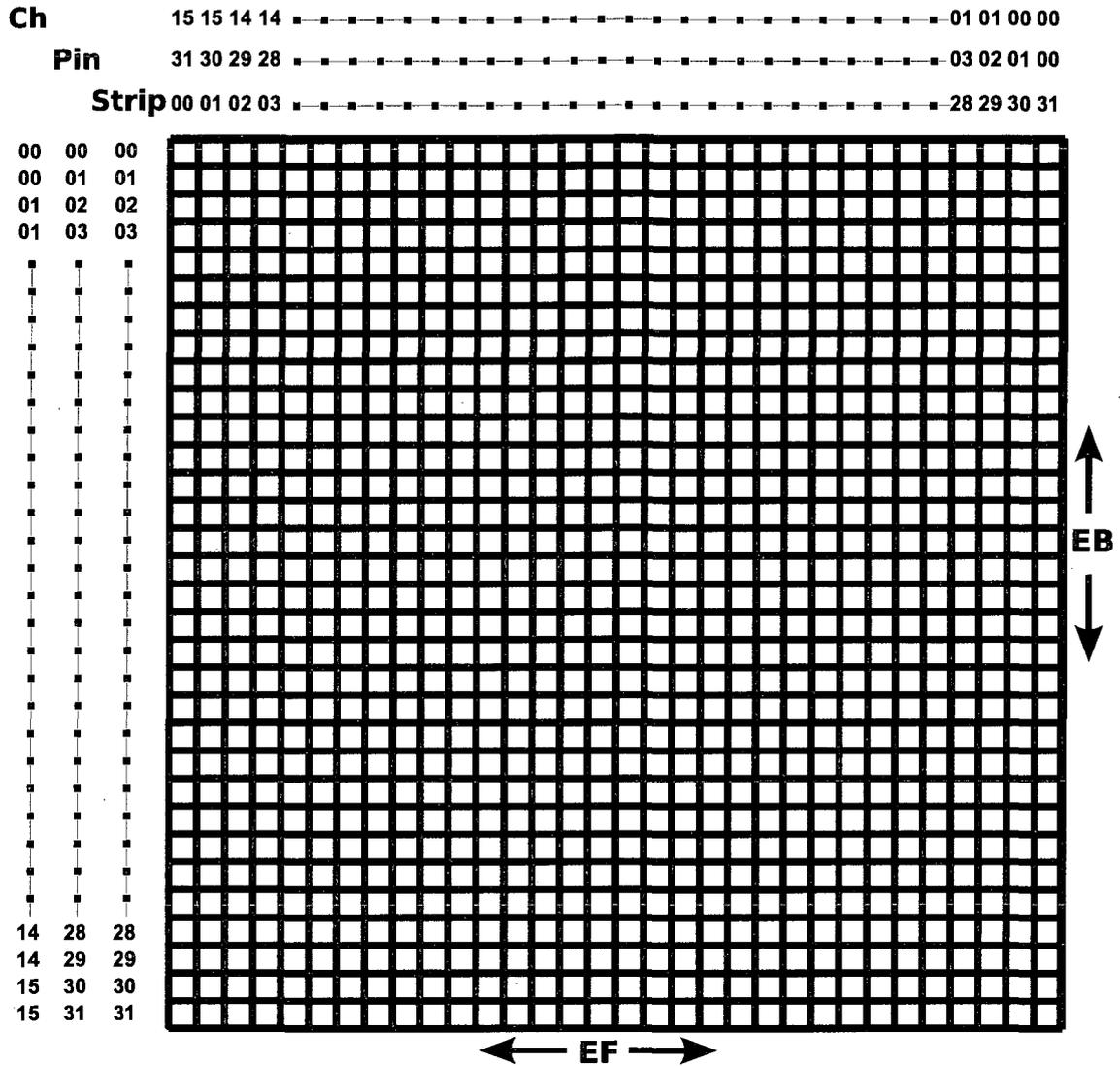
Figure 3.5 – Diagram of the chip/channel/strip mapping for the HiRA DSSD.
