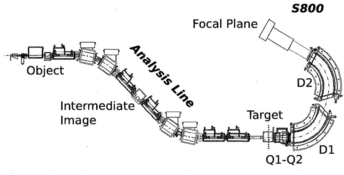
Figure 2.4 – S800 analysis line and spectrograph.
