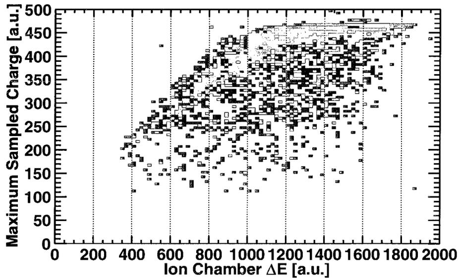
Figure 3.27 – Saturation of CRDC 2 pad 52.
