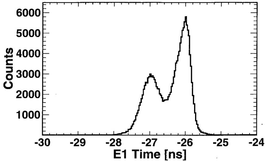
Figure 3.24 – Timing signal for the E1 scintillator.
