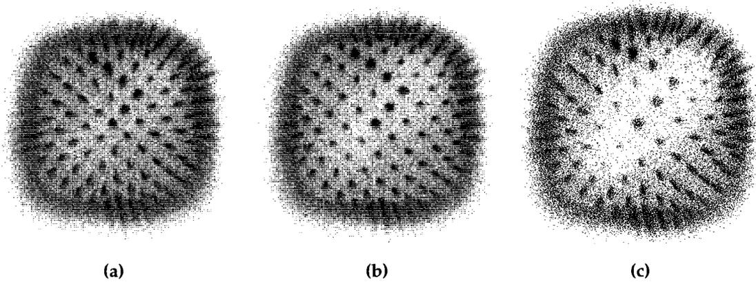
Figure 3.19 – MCP 1 mask pattern for (a) pedestal values  $-10$  channels, (b) pedestal values  $0$  channels, and (c) pedestal values  $+10$  channels.
