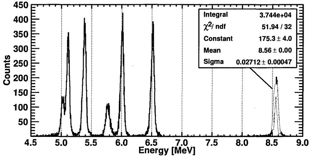
Figure 3.4 – Telescope 9  $^{228}\text{Th}$   $\alpha$ -source calibration for all front strips of the DSSD.
