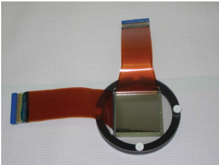
Figure 3.15: Photograph of a HiRA double-sided silicon strip-detector (E) in a circular plastic container. The two brown bands extending outside the container are the signal cables.
