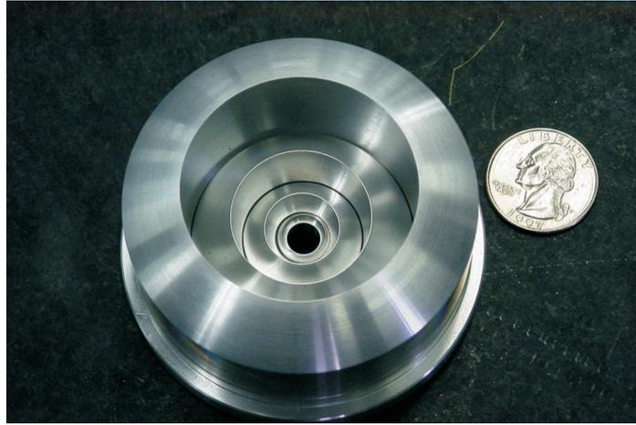
Figure 4.4. Photograph of spherical electrodes used to focus ions into extraction nozzle.
