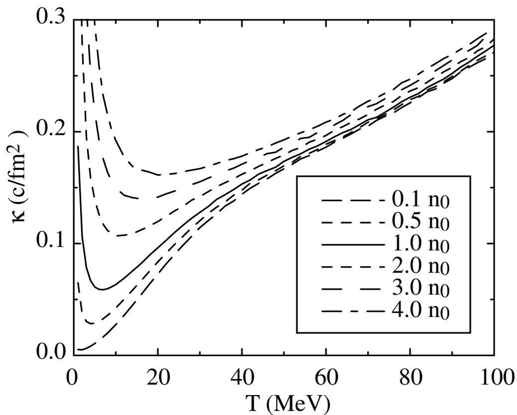
Figure 4.3: Thermal conductivity  $\kappa$  in symmetric nuclear matter, at different indicated densities in units of  $n_0$ , as a function of temperature  $T$ . The conductivity increases as density increases.
