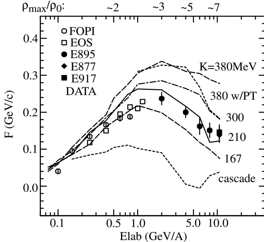
Figure 1.3: The flow parameter  $F$  as a function of energy. The symbols represent the experimental result for sideward flow at different energies. The lines are theory prediction for the flow, and different equation of states are labelled by their corresponding compressibility value. (from [7]).
