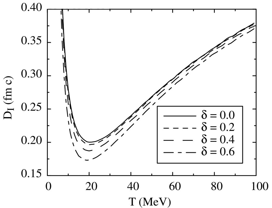
Figure 4.2: Isospin diffusion coefficient  $D_I$  at normal density  $n = n_0 = 0.16 \text{ fm}^{-3}$  and different indicated asymmetries  $\delta$ , for  $U_i = 0$ , as a function of temperature  $T$ . An increase in the asymmetry generally causes a decrease in the coefficient, as discussed in the text.
