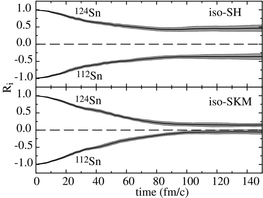
Figure 5.13: The isospin diffusion ratio as defined by Eq. (5.6) is plotted as a function of time for two IEOS. The top panel is for the most stiff symmetry energy density dependence (iso-SH), and the lower panel is for the most soft symmetry energy density dependence (iso-SKM). Note the stability of the ratio after 100 fm/c. The shaded areas around the lines indicate the statistical error from averaging over multiple simulations.
