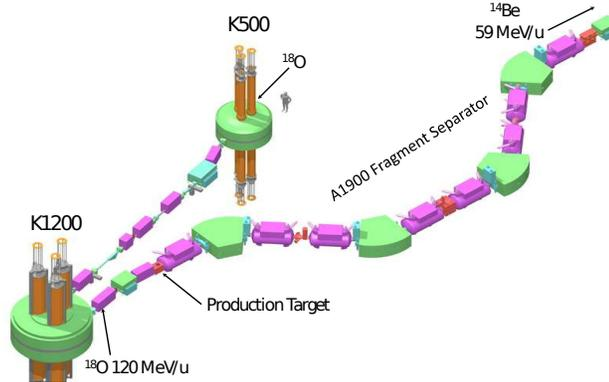
Figure 2.1: Diagram of the beam production mechanism. The primary beam of  $^{18}\text{O}$  is accelerated through the K500 and K1200 until it reaches an energy of 120 MeV/u and strikes a  $3196 \text{ mg/cm}^2$  beryllium target. The A1900 fragment separator then selects  $^{14}\text{Be}$  fragments from other reaction products.
