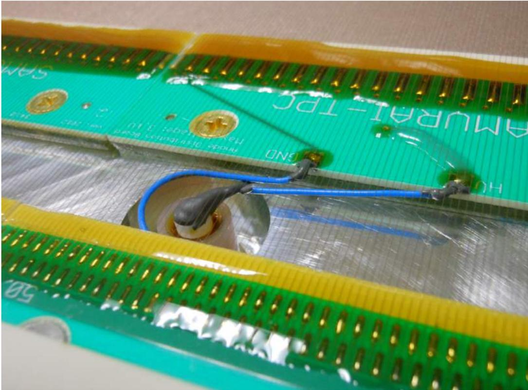
Figure 2.66: Insulate the anode plane connections
