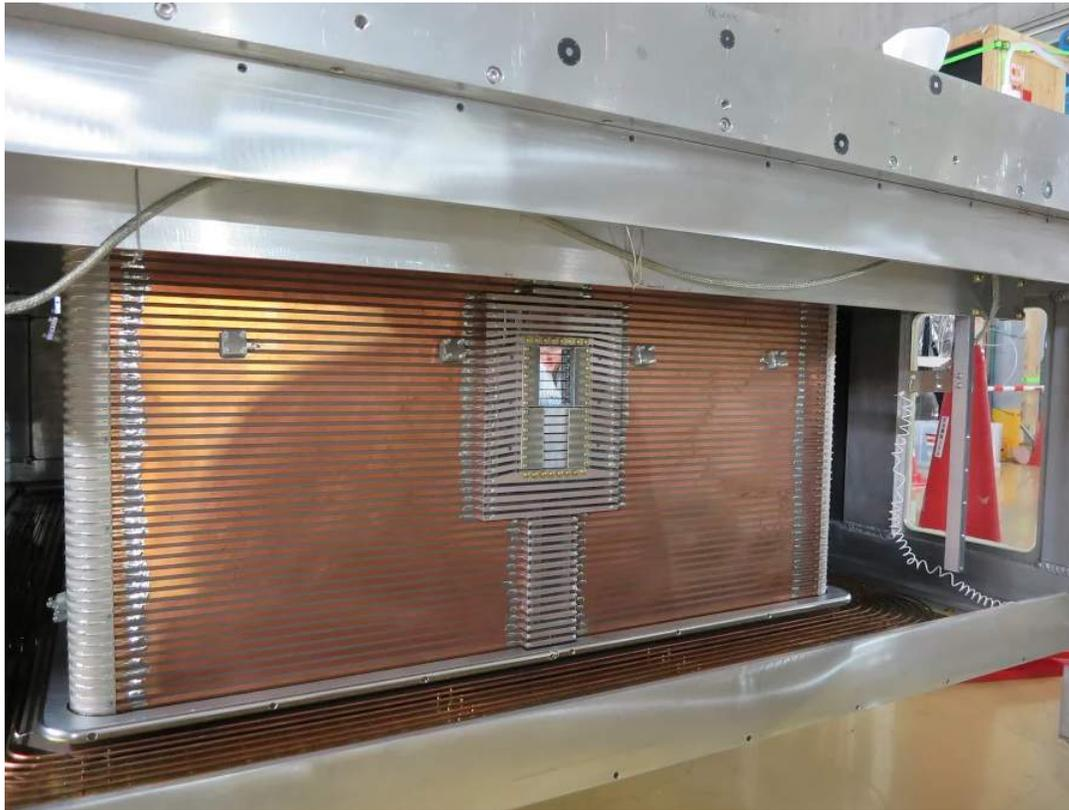
Figure 2.89: The S $\pi$ RIT TPC without a target mechanism
