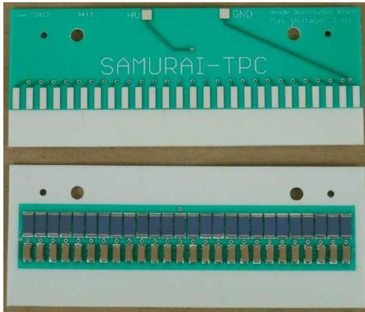
Figure 2.54: The printed circuit board (PCB) for anode wires: 26 pads are connected to the high voltage by 26 of 10 M $\Omega$  resistors (blue). Each pad is connected to an external ground by 1 nF capacitor (brown).
