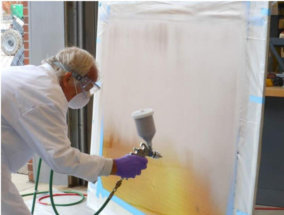
Figure 2.75: Conductive paint was applied at the center of the polycarbonate sheet.
