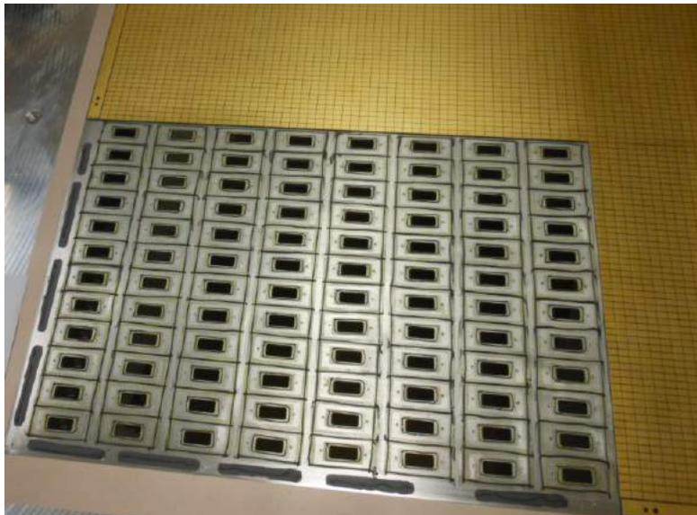
Figure 2.45: Gluing pattern for the pad plane
