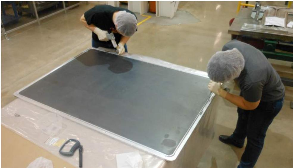
Figure 2.27: Prepare the cathode for gluing.
