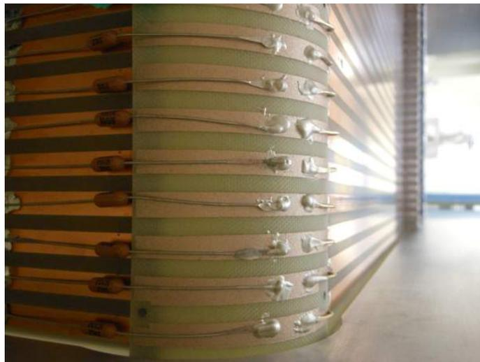
Figure 2.30: Insert  $1\text{ k}\Omega$  resistors along the strips.
