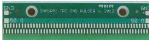
Figure 2.55: Printed circuit board for ground plane
