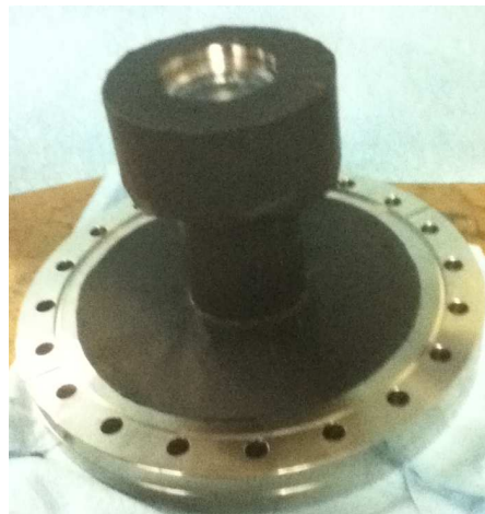
Figure 4.7: Photograph of the inverted viewport window flange covered in black aluminum foil.
