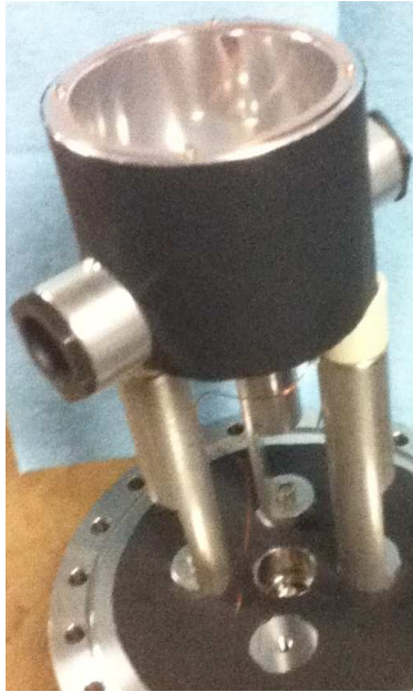
Figure 4.4: Photograph of the ellipsoidal reflector covered in black aluminum foil.
