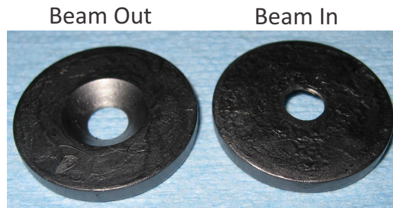
Figure 3.6: Photograph of two 7 mm inner diameter beam line apertures after being painted with graphite paint to be conductive.
