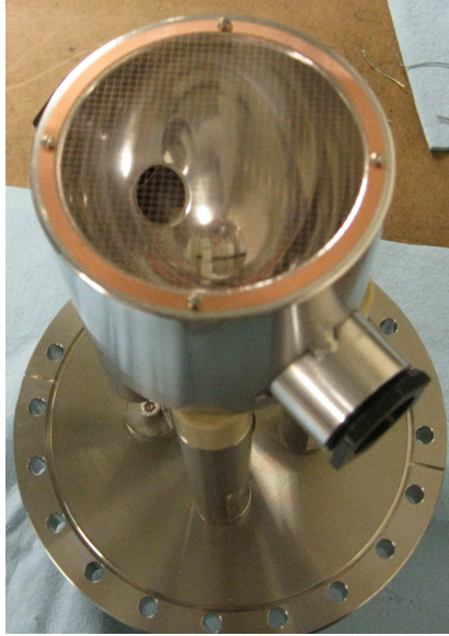
Figure 3.4: Photograph of the ellipsoidal reflector after hand polishing.
