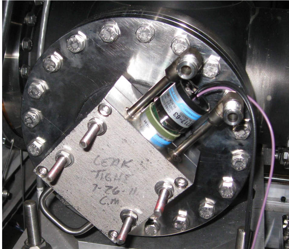
Figure 3.12: A photograph of the “red” photon detection system PMT enclosure attached to the photon detection system vacuum chamber.
