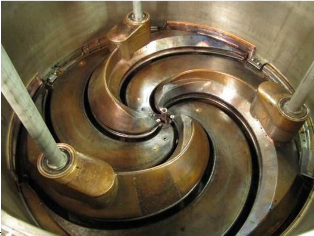
FIGURE 4.1. Internal view of an NSCL cyclotron. Usually the equipment is under high vacuum, and must be temporarily taken off line to view its internal structure [37].
