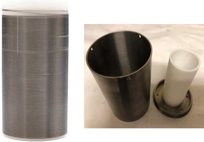
Figure 5.16: 600  $\mu\text{H}$  NbTi inductor coil (left) and NbTi inductor case (right) used for the high-Q SIPT FT-ICR detection circuit. The inductor coil consists of 194 turns of 250  $\mu\text{m}$  NbTi wire with tubular Teflon coating wrapped around a Teflon core. The windings were then covered by an additional layer of Teflon tape, which provides both mechanical support and some additional amount of thermal conductivity.
