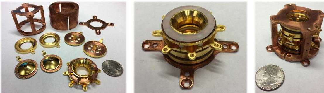
Figure 5.7: SIPT Penning trap electrodes before assembly (left), partway through assembly (middle) and after assembly (right).
