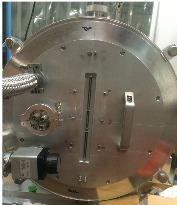
Figure 3.3: Photograph of Flange On the left are the two gas inlets, for the active and insulating volumes (outlets are positioned elsewhere) flanking high voltage feedthroughs for powering the Micromegas and last ring (see text). The long vertical slit is the connector where the GET electronics attach to the detector.
