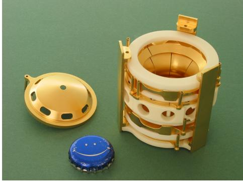
Figure 3.6: The LEBIT Penning trap, shown here with one endcap removed and a bottle cap for scale.
