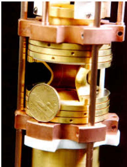
Figure 6.5: The Canadian Penning Trap (CPT), shown here with a Canadian gold dollar for scale.
