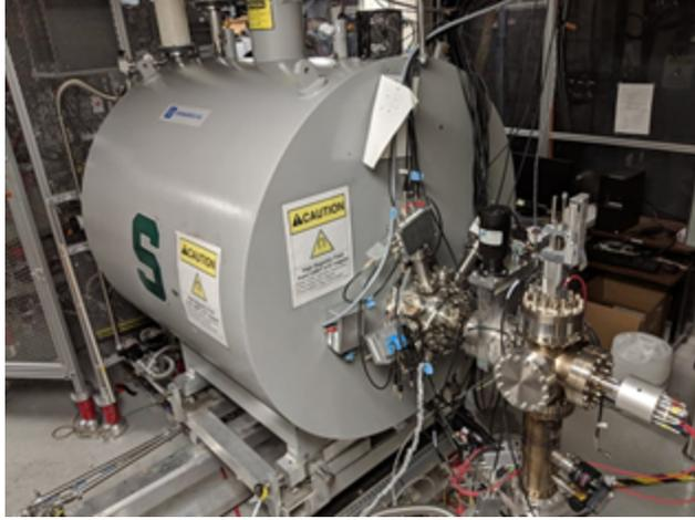
Figure 3.10: The LEBIT magnet, a 9.4 Tesla superconducting solenoid.
