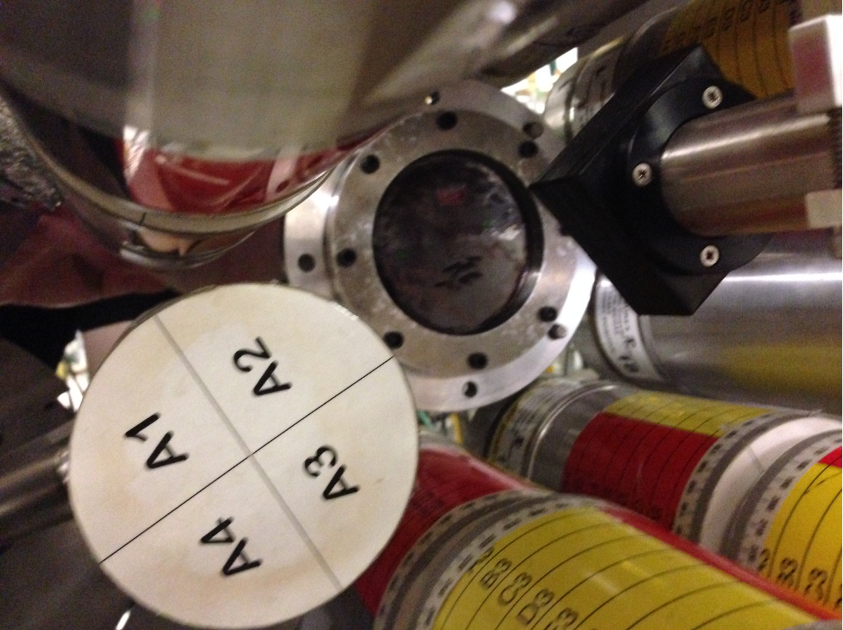
Figure 3.5: The secondary beam exits through a thin kapton window after which it travels 20 cm in air before implanting into the EJ200 plastic scintillator.
