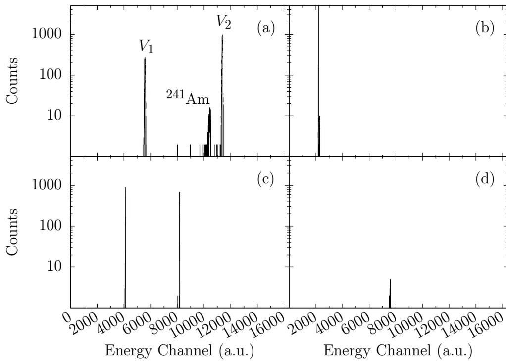
Figure 3.4: Spectra from silicon detector calibrations. (a) shows a normal channel with a  $^{241}\text{Am}$  peak and two pulser peaks. (b) shows a channel with only one pulser peak. (c) shows a channel with no  $^{241}\text{Am}$ . (d) shows a channel with no pulser peaks.
