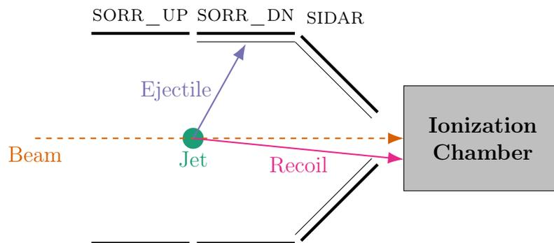
Figure 2.7: A diagram of the detectors used in the experiment and the reaction products they detect.
