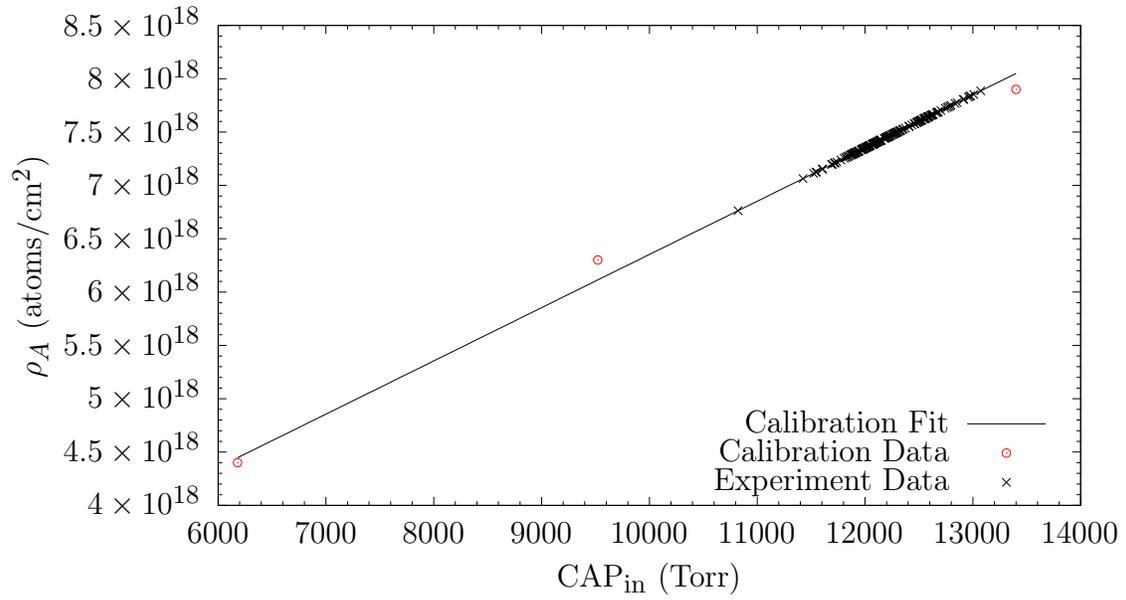
Figure 3.19: The relationship between the target areal density and the pressure measured at CAP<sub>in</sub>. The circles are the calibration points, and the crosses are the experimental values that were calibrated using this fit.
