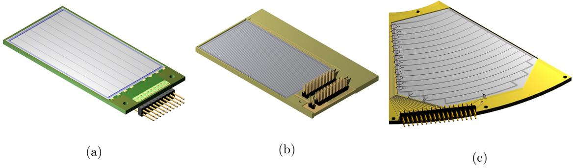
Figure 2.10: The silicon detectors used in this experiment are (a) 4 60  $\mu\text{m}$ -thick Micron BB10s, (b) 12 1 mm-thick Micron BB15s, and (c) 5 60  $\mu\text{m}$ -thick and 5 1 mm-thick Micron YY1s.
