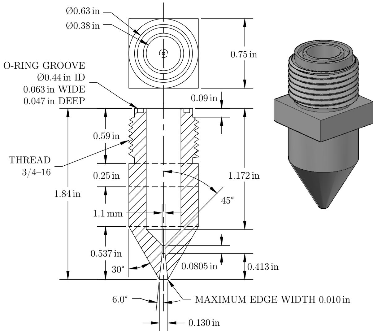
Figure 2.5: The nozzle used in this experiment.
