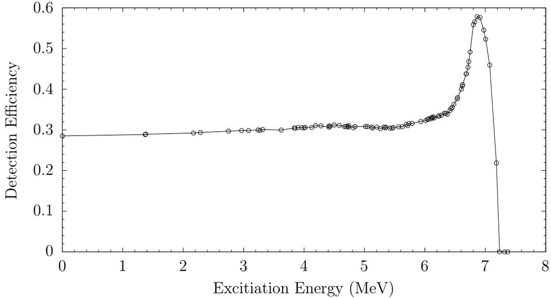
Figure 3.17: The detection efficiency as a function of recoil excitation energy for the  $^{34}\text{Ar}(\alpha,\text{p})^{37}\text{K}$  reaction. The total detection efficiency is an average of the efficiencies of each level weighted by the relative cross section of the levels.
