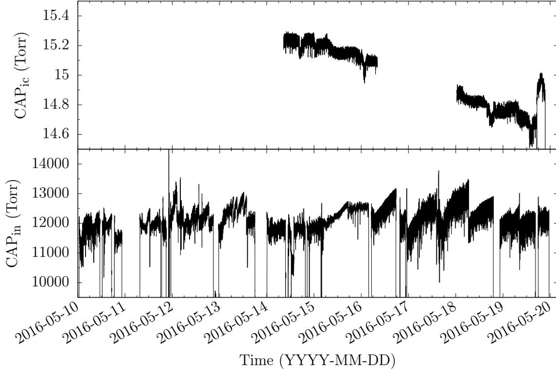
Figure 3.6: The time series data for the pressures measured by  $CAP_{ic}$  and  $CAP_{in}$ .  $CAP_{ic}$  measured the pressure in the ionization chamber; for parts of the experiment, it was not recorded by the EPICS system. Hand measurements were still recorded during this time, but these were not used for the calibration.  $CAP_{in}$  measured the pressure immediately before entering the nozzle; this was used to determine the areal density of the jet.
