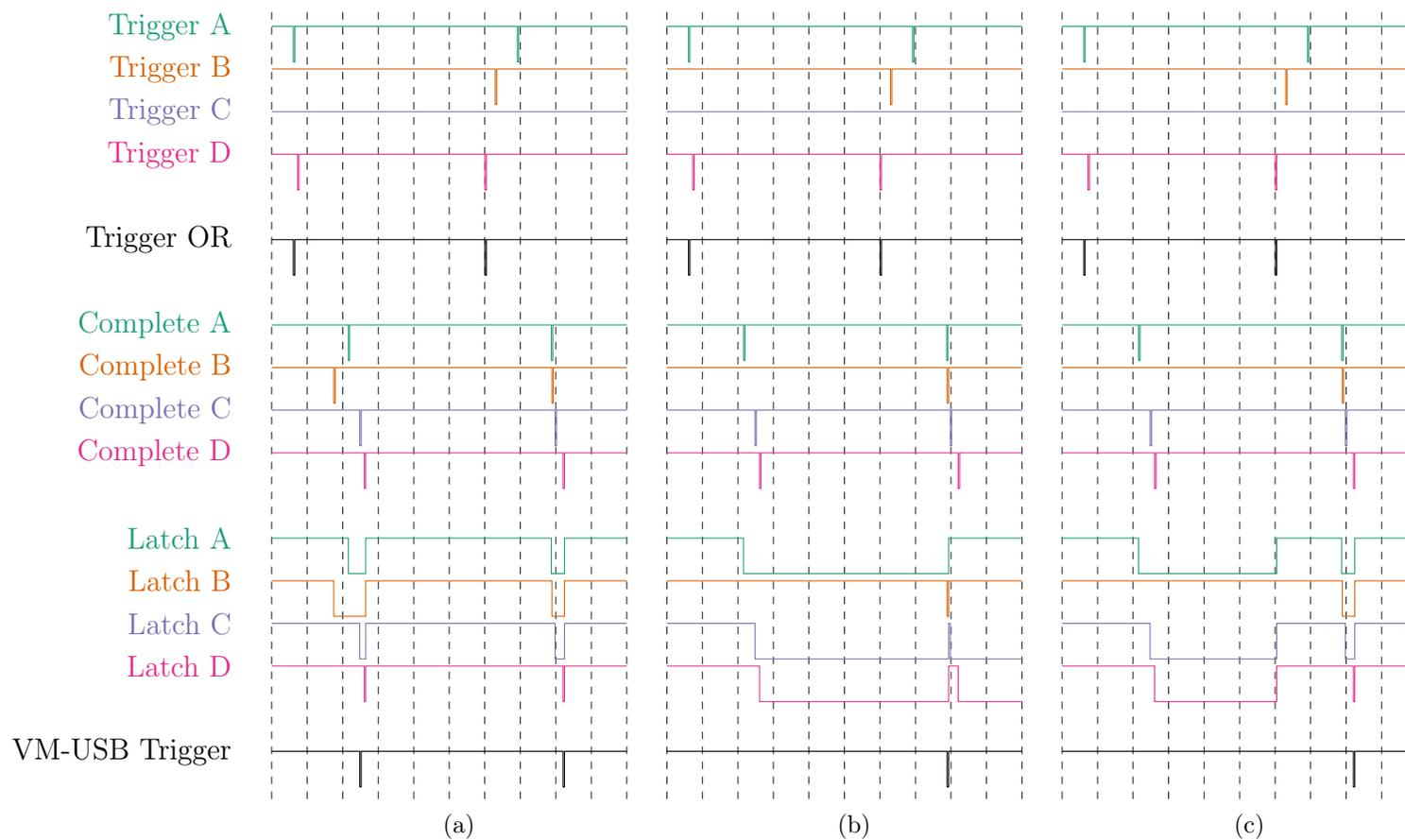
Figure 2.13: An example showing how the four ASICs motherboard triggers are combined to create the VM-USB trigger. (a) shows two events during normal operation. (b) shows how a missing complete signal can propagate errors to subsequent events. (c) shows how the OR of the motherboard triggers can be used to prevent this error from propagating to other events.
