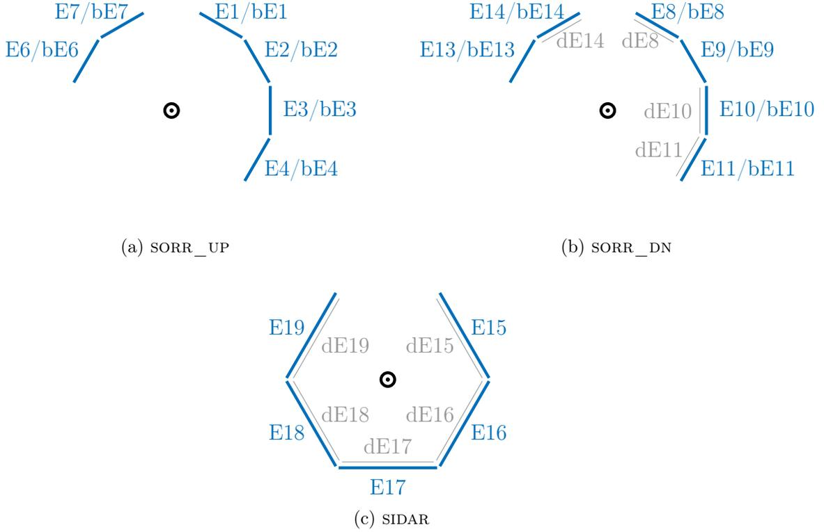
Figure 2.9: The silicon detector array used in this experiment, looking upstream, toward the source of the beam. The detector naming counts up going clockwise, starting at the upstream section and repeating for each subsequent downstream section. Detectors 5 and 12 were removed to accommodate jet and beam tuning hardware.
