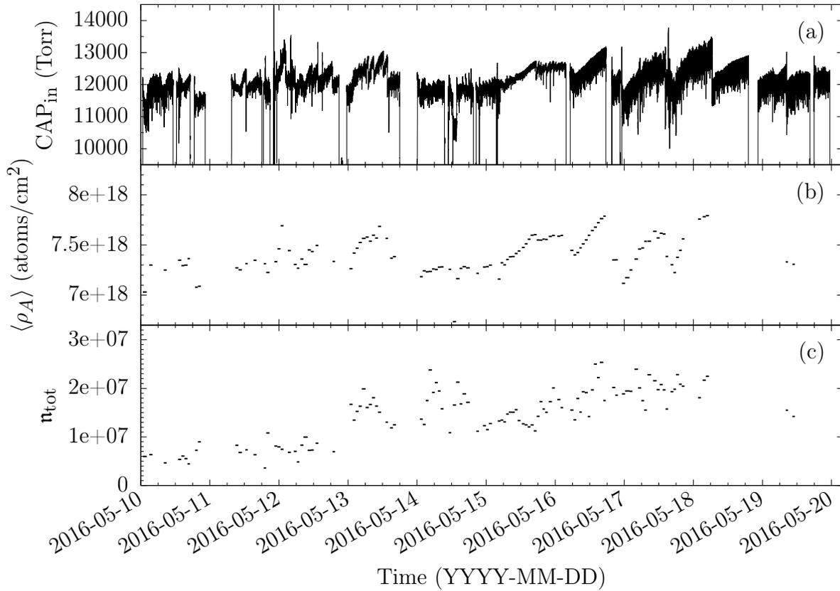
Figure 3.20: The time series data that changes for each run. (a) shows the continuous data for  $CAP_{in}$  throughout the entire experiment. (b) shows the areal jet density averaged over the time span of each run. (c) shows the total number of particles delivered to the target for each run.
