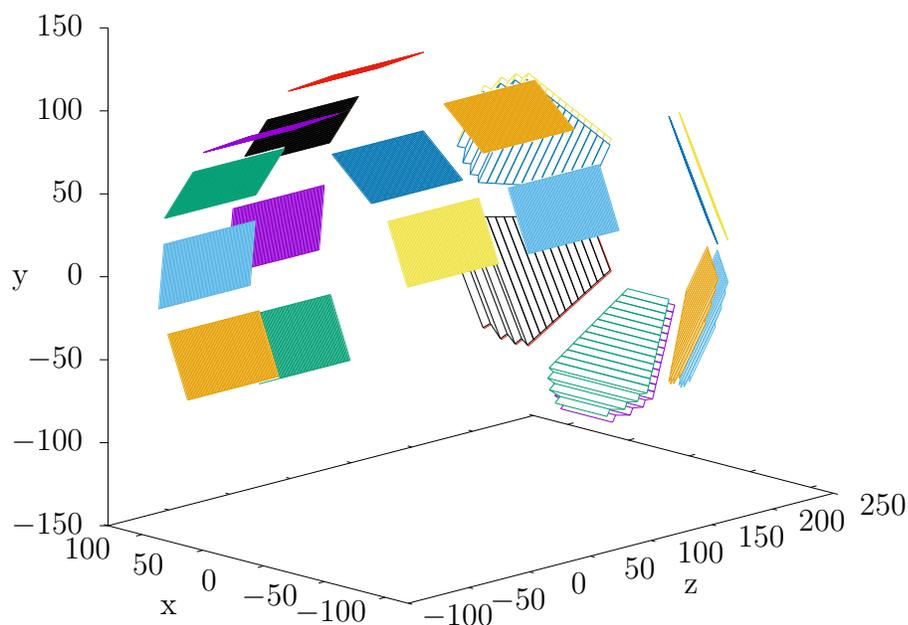
Figure 2.11: The positions of the silicon detectors in the experiment. The  $z$ -axis is the beam axis and the  $y$ -axis is the jet axis, meaning the reaction location is at the origin.
