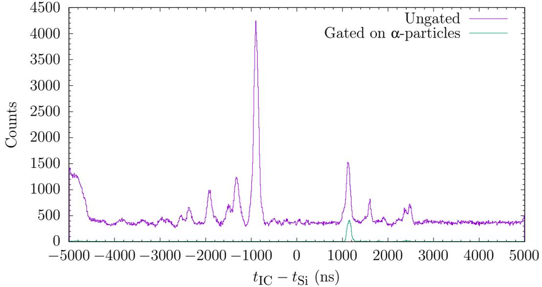
Figure 3.9: The time difference between hits in the ionization chamber and the silicon detectors. “Ungated” shows this for all hits. “Gated on  $\alpha$ -particles” shows this only for hits in E9 and E13 inside the  $\alpha$ -particle gate shown in Figure 3.10.
