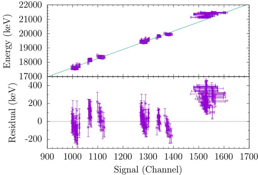
Figure 3.8: The calibration curve for the E section of the ionization chamber. The lowest energy group corresponds to  $^{34}\text{Ar}$ , the middle  $^{34}\text{Cl}$ , and the highest  $^{34}\text{S}$ . The  $^{34}\text{S}$  points do not agree with the  $^{34}\text{Ar}$  and  $^{34}\text{Cl}$  points. This is likely due to interference from the larger  $^{34}\text{Cl}$  peak.
