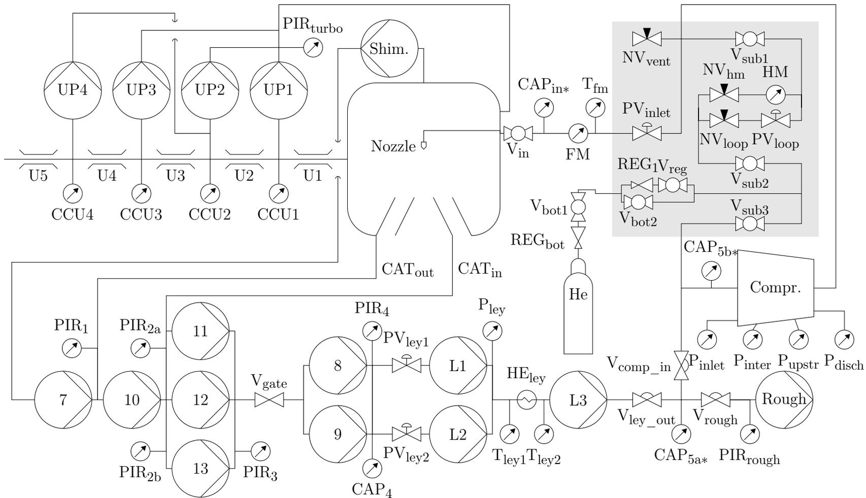
Figure 2.3: Diagram of the JENSA gas system.
