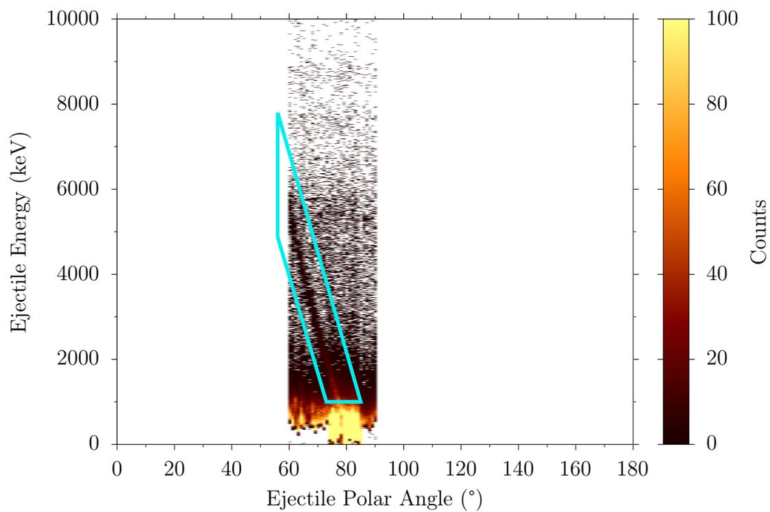
Figure 3.10: The energy-polar angle relationship in E9 and E13, the detectors without a thin detector in front of the thick detectors. These detectors can clearly see the  $\alpha$ -particles from elastic scattering. A gate is drawn around these hits and used as the gate in Figure 3.9.
