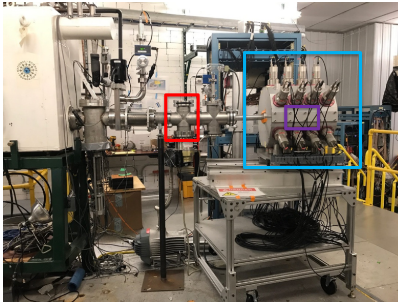
Figure 2.2: A picture of the e14505 setup in the S2 vault. SuN is shown on the right in the large blue box, the DSSD and veto and located in the center of SuN (indicated by the purple box), and the PIN detectors are located upstream of SuN in the red box.
