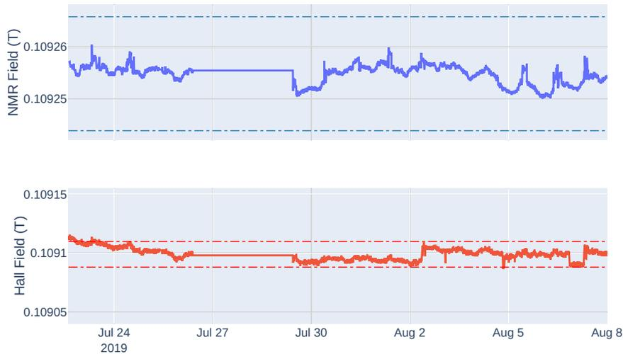
Figure 4.6: Dipole B1 magnetic field long term stability test as measured with NMR (top) and Hall probe (bottom). The dot-dashed lines correspond to  $\pm 0.01\%$  stability levels. The flat lines between July 26 and July 29 correspond to a control system connection drop.
