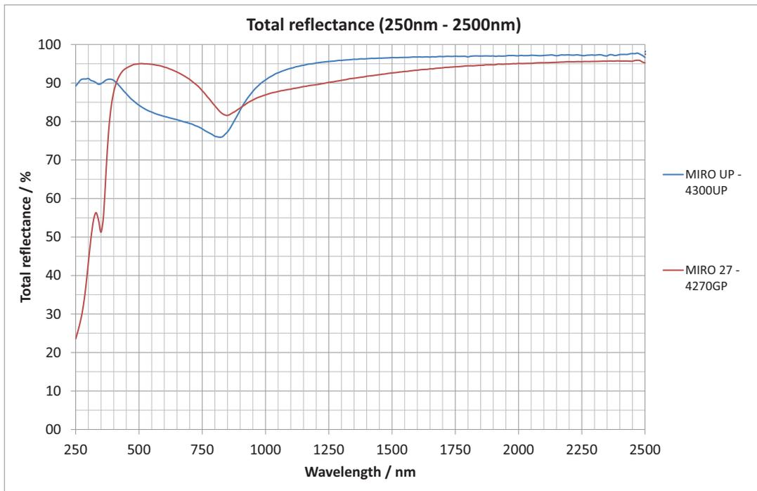
Figure A.8: Reflection data for the aluminum sheeting used for the reflective surfaces of the new PDS. The MIRO 4300UP was used, in order to allow for good reflectivity throughout the UV range (250–450 nm).
