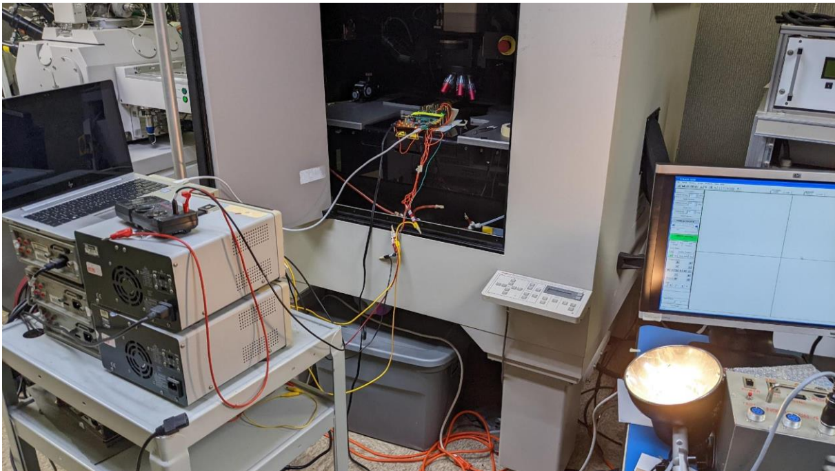
Figure 17: Photograph of the ADS9818 latchup replication test setup.
