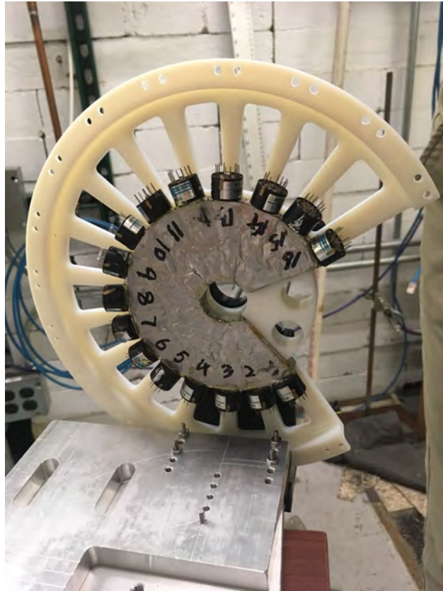
Figure 2.19 A picture of the Forward array (FA). The FA consists of 18 annulus sectors, numbered using marker pen from 1 to 16; the remaining two wider sectors are not labeled. Photo courtesy of J. Barney.
