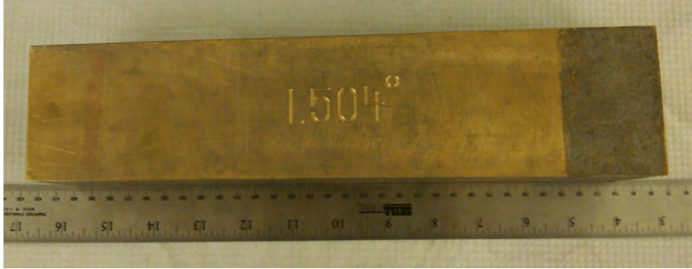
Figure 5.1 A photograph of one of the shadow bars, taken with a ruler placed next to it for scale. Adapted from [184].
