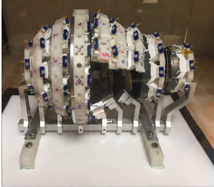
Figure 2.6 A photograph of the Microball taken after the teardown of the experiment. Some rings and scintillators are placed back to their original positions before storage, e.g. Ring 6.
