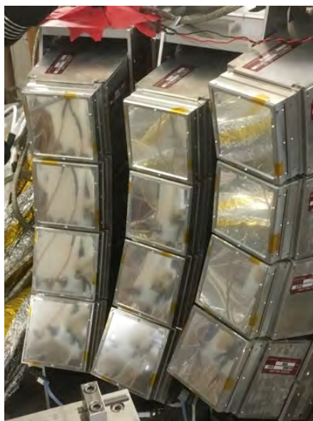
Figure 2.12 A photograph of HiRA10 array taken during the preparation of the experiment. There are a total of 12 telescopes, arranged in three vertical columns, called “towers”, each consists of four telescopes.
