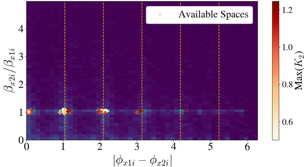
Figure 4.30 2D Histogram of optimum lattice locations where the compensating  $K_2$  coefficients with the two new sextupoles are minimized with available drift spaces candidates scattered on top of it.
