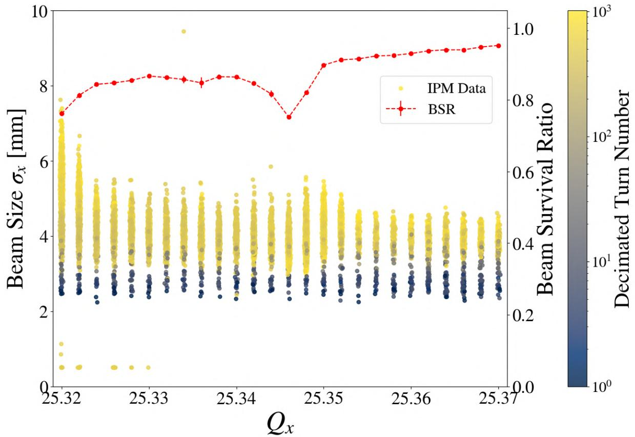
Figure 6.7 Static tune scan at an equivalent intensity of 14 Booster turns or approximately  $4.5 \times 10^{10}$  ppb.
