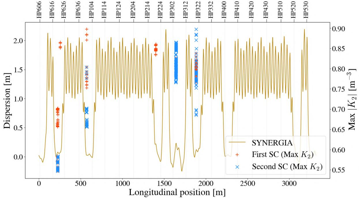
Figure 4.31 Dispersion function of the Recycler Ring with possible new locations to introduce a pair of sextupole magnets that cancel out  $h_{3000}$  and  $h_{1020}$  simultaneously. The right y-axis shows the maximum compensation  $K_2$  coefficient needed with these new candidates.
