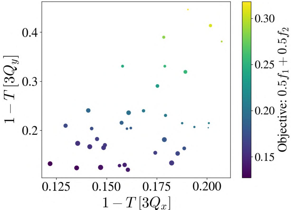
Figure 4.19 Multiobjective Nelder-Mead optimization of the transmission through  $3Q_x$  and  $3Q_y$ . The objective function to be minimized was defined as an equally weighted sum of both minus transmissions—corresponding to the fractional losses through the resonance lines.
