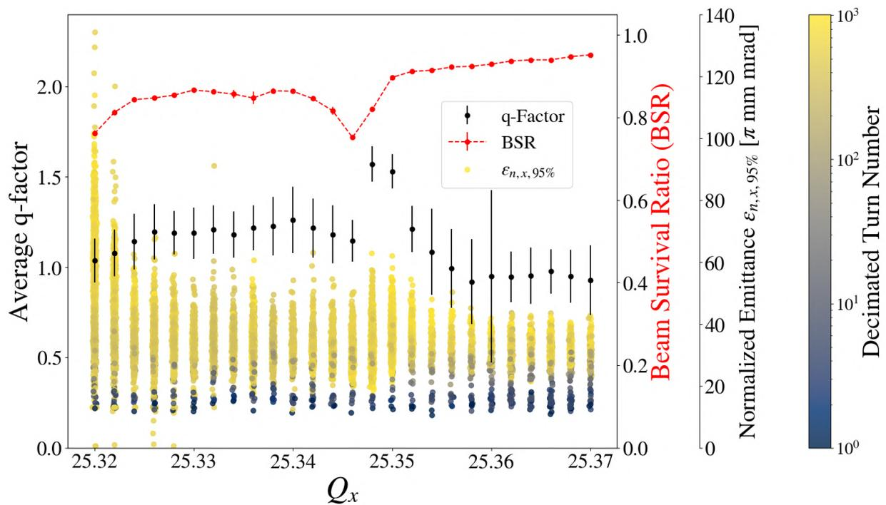
Figure 6.11 Static tune scan with beam survival ratio (BSR), average  $q$ -factor for the  $q$ -Gaussian fits, and normalized emittance at an equivalent intensity of 14 Booster turns or approximately  $4.5 \times 10^{10}$  ppb.
