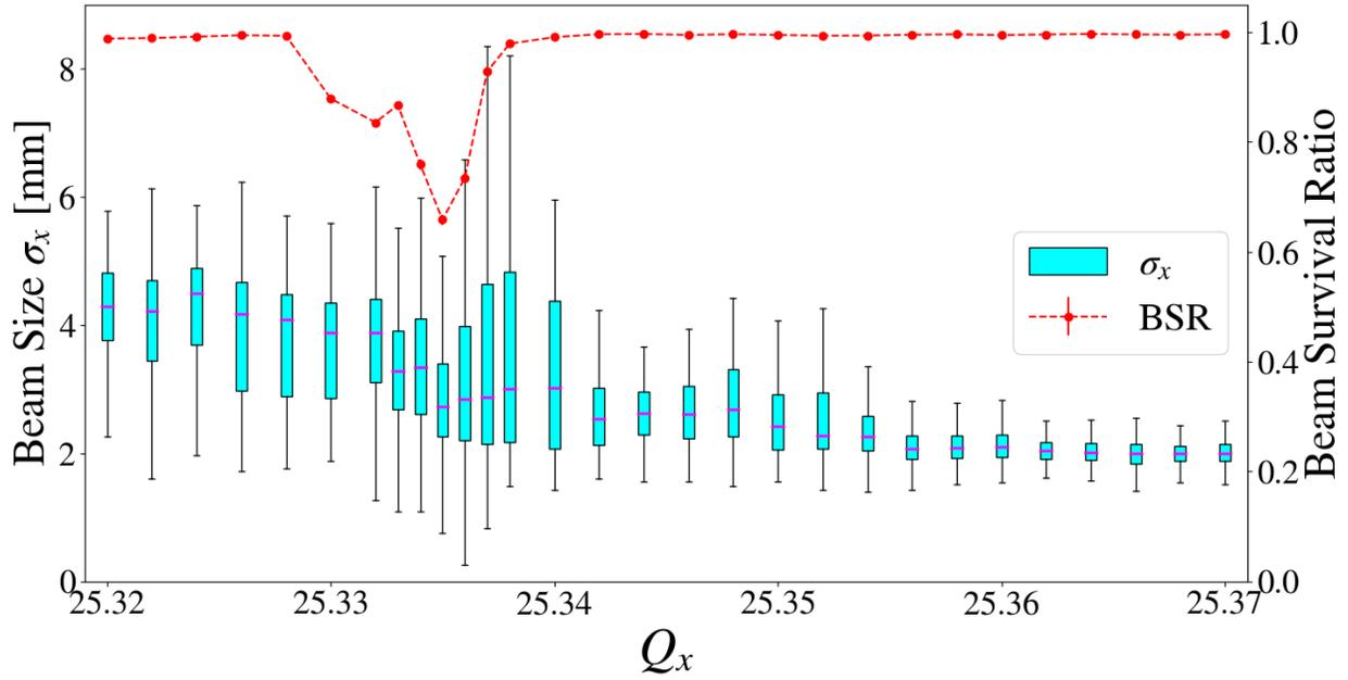
Figure 6.12 Static tune scan with beam survival ratio and IPM data box plots with  $3Q_x$  compensation, transverse dampers ON and 2 Booster Turns of equivalent intensity or approximately  $0.5e10$  ppb.
