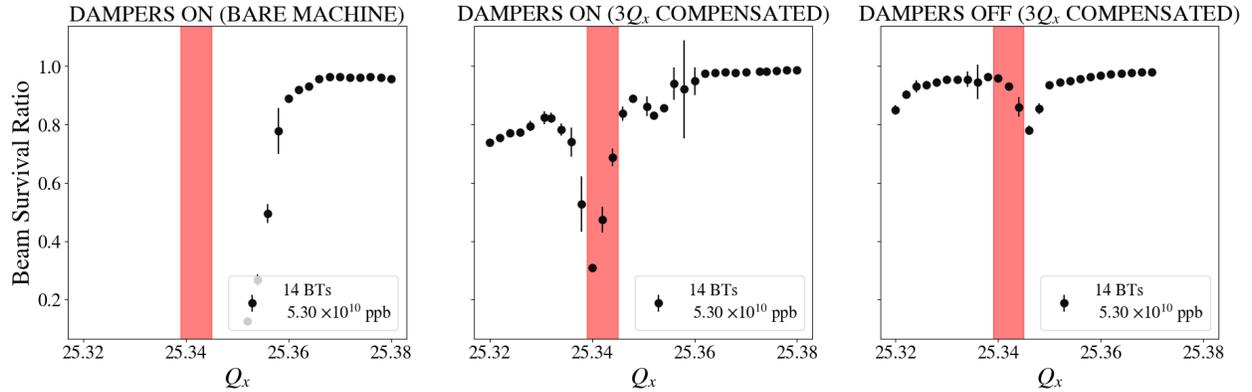
Figure 7.1 Transverse damper effect on resonance compensation for bare machine + dampers ON,  $3Q_x$  compensated + dampers ON, and  $3Q_x$  compensated + dampers OFF configuration. The red band corresponds to the  $3Q_x$  stop band at an intensity of 0.5 ppb with dampers ON.
