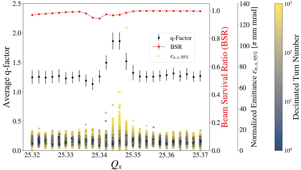
Figure 6.9 Static tune scan with beam survival ratio (BSR), average  $q$ -factor for the  $q$ -Gaussian fits, and normalized emittance at an equivalent intensity of 2 Booster turns or approximately  $0.5 \times 10^{10}$  ppb.
