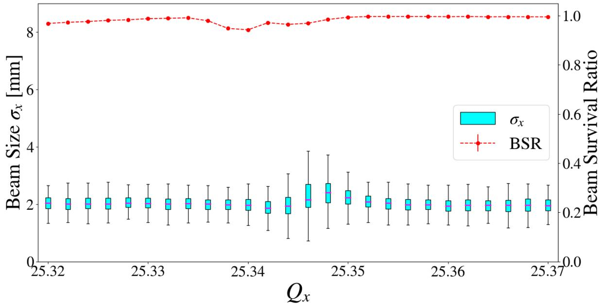
Figure 6.13 Static tune scan with beam survival ratio and IPM data box plots with  $3Q_x$  compensation, transverse dampers OFF and 2 Booster Turns of equivalent intensity or approximately  $0.5e10$  ppb.
