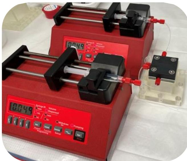
Figure 43: A fully assembled SLM extraction with two syringe pumps.
