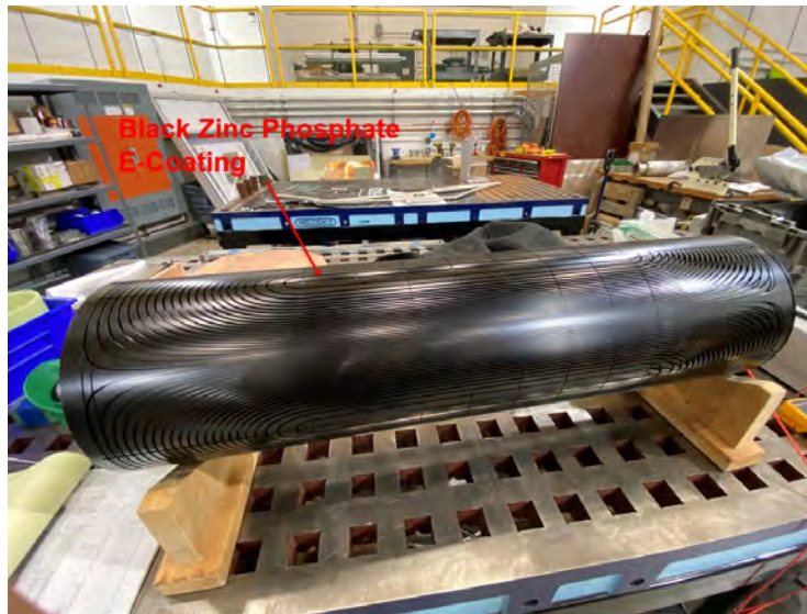
Figure 4.7 Winding bobbin after electro deposition of zinc phosphate "e-coating" completion, the bobbin is then placed on the winding table for real winding of quadrupole.
