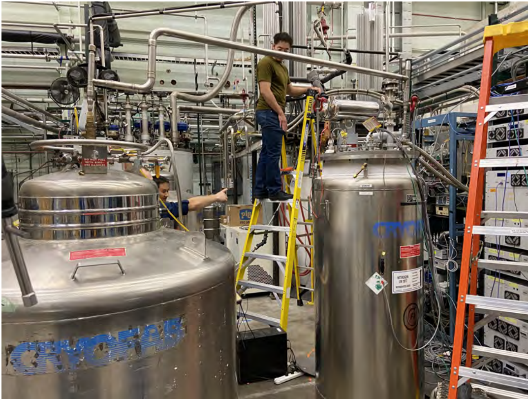
Figure 5.21 Picture of 1000 liter liquid helium Dewar connected to the coil testing Dewar via liquid helium U-tube transfer line.
