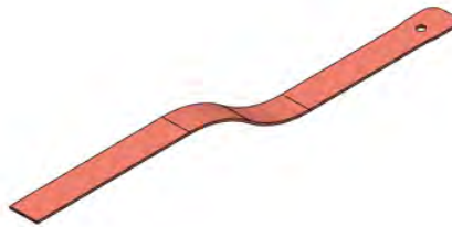
Figure 5.5 Model of copper current lead design. Copper lead is designed with a length of 250 mm and cross sectional area of 25.8 \text{ mm}^2 .
