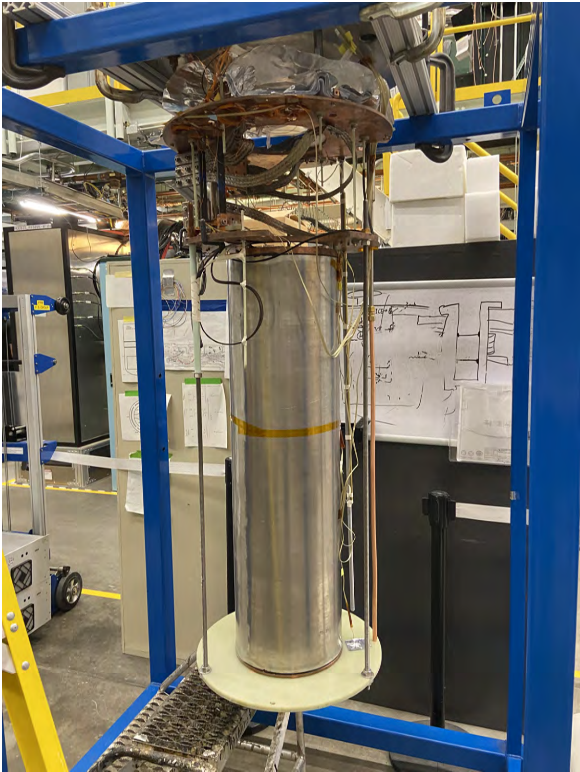
Figure 5.17 Picture of the full coil testing assembly ready for insertion into testing Dewar for liquid Helium testing.
