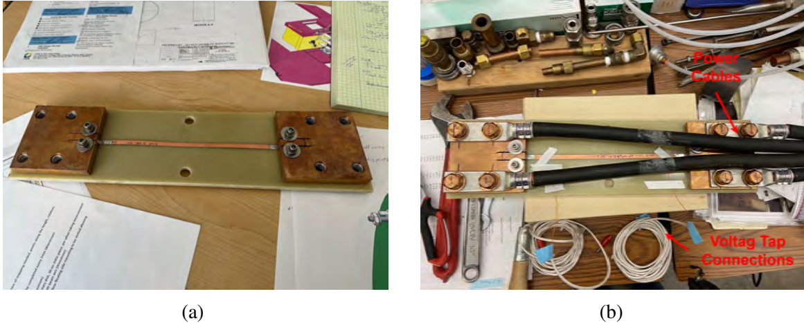
Figure 5.6 a) ReBCO tape soldered to copper terminals for power supply connection and mounted to G10 plate. b) ReBCO testing with power leads connected to terminals and voltage taps connected to ReBCO tape sample.
