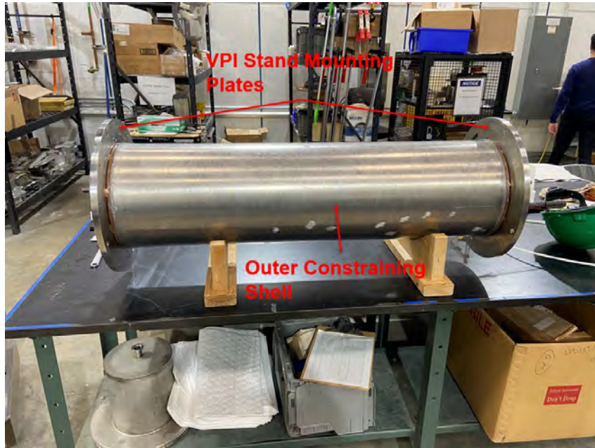
Figure 4.18 Picture of CDQ single layer coil fully prepared for vacuum impregnation [29].
