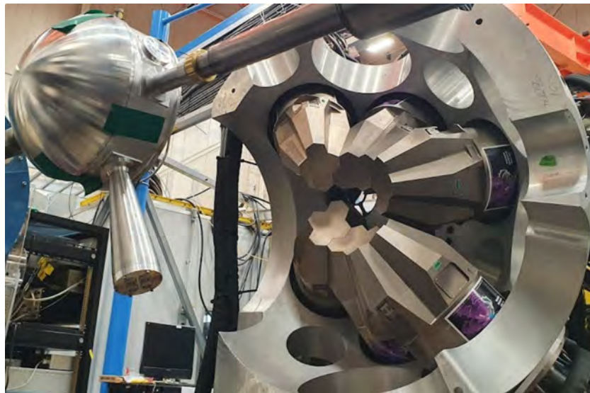
Figure 3.6: Photograph of an open hemisphere of GRETINA with 6 modules visible. The slots in the frame into which the modules are mounted can be seen, as well as the tight configuration of the crystals. This hemisphere may be closed with the one out of view of the picture so that the crystals surround the target chamber.
