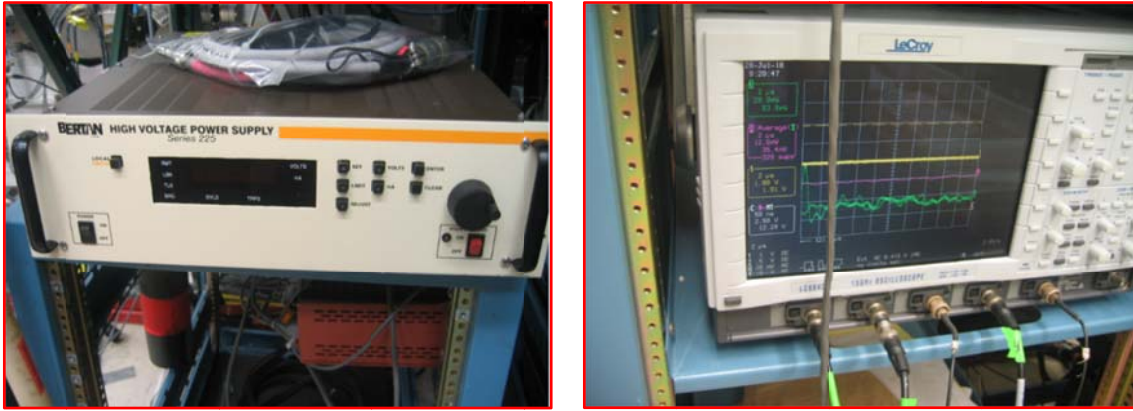
Figure 6.5: High voltage power supply (BERTAN 225) for the retarding grid (left) and oscilloscope (LeCroy LC684DXL) (right).
